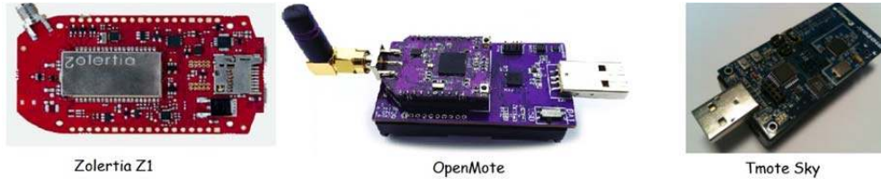
Figure 1.2. Different types of constrained devices (Development tools Archives, n.d.; Vilajosana, Tuset, Watteyne, & Pister, 2015; Insense Examples, n.d.)
