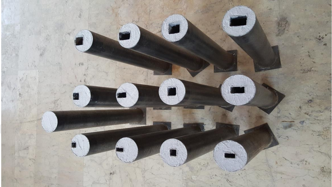
Figure 3.7 The gap filled with epoxy after curing period.
