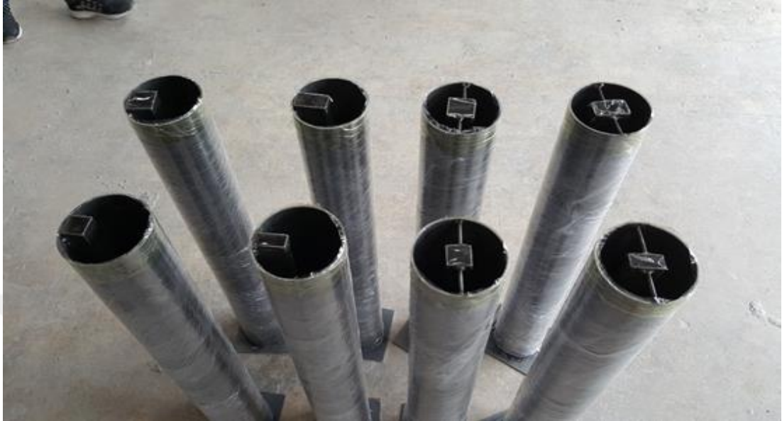
Figure 3.5 The specimens before casting.
