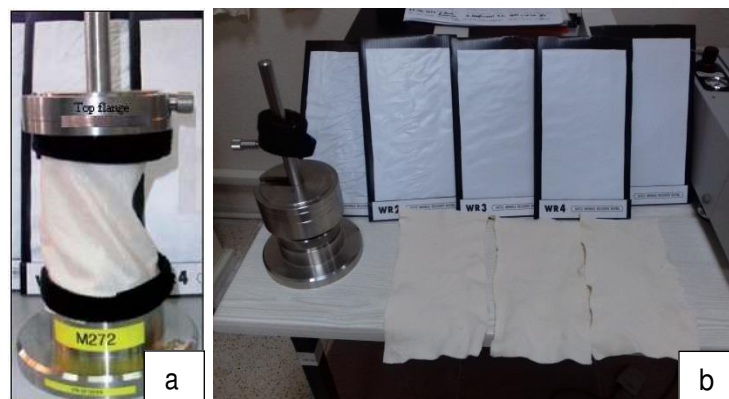
Figure 3.46 Wrinkle recovery tester and sample pictures and comparison of fabrics
