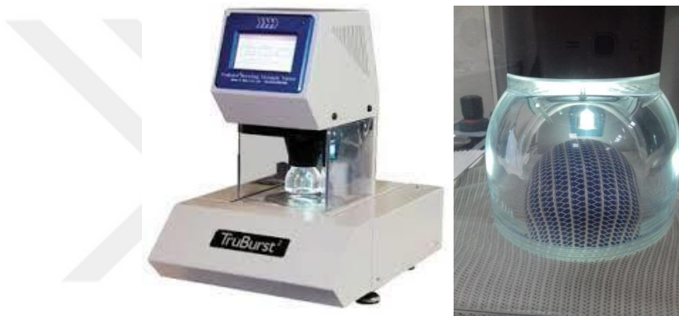
Figure 3.41 Bursting strength image of tester and fabric burst moment
