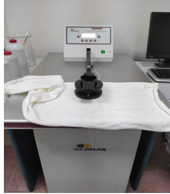
Figure 4.11 Air permeability measurement tester
