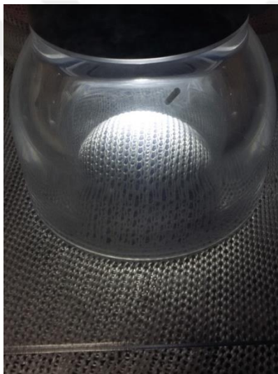
Figure 4.15 Tested specimen for bursting strength when diaphragm was inflated
