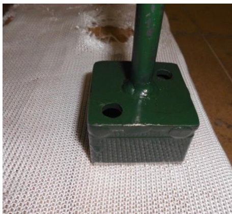
Figure 4.9 A measurement of areal density with die cutter
