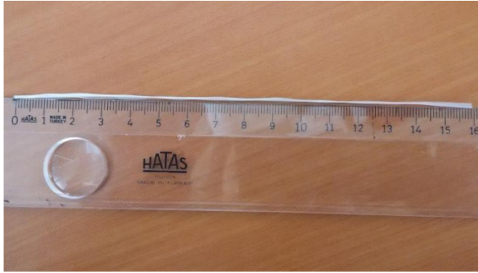
Figure 4.13 Measured loop lengths by ruler
