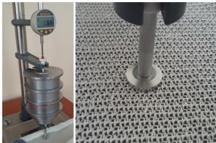
Figure 4.7 An example of the tested fabric during thickness measurement
