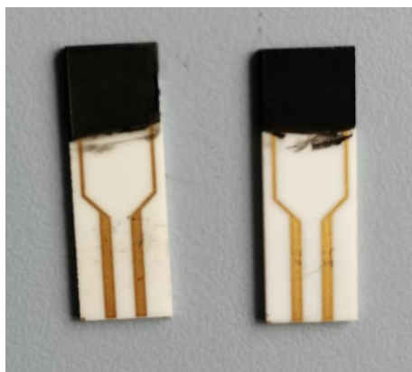
Figure 2-3 : Spin coated interdigitated electrodes for gas sensing
