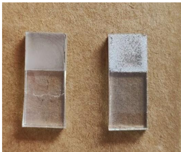
Figure 3.32. Thin films of pristine materials before proton exchange (left), after proton exchange (right)
