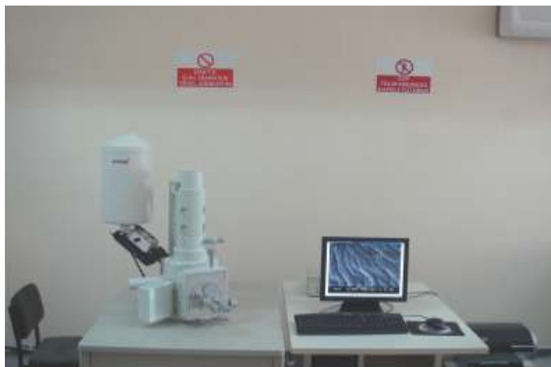
Figure 5.2 Scanning electron microscopy (Jeol JSM-6060) coupled with EDS system.
