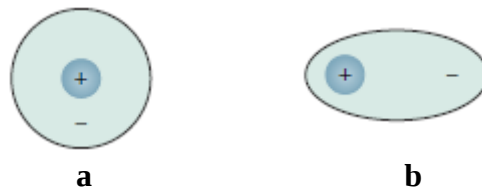
Figure 4.8 Electric dipoles scheme a. unpolarized b. polarized
