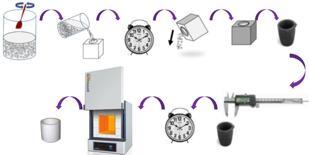
Figure 4.2 Basic steps of hollow slip casting (Personal archive, 2018)
