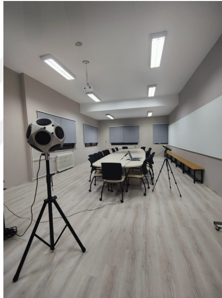
Figure 21. In-situ measurement instruments in the classroom
