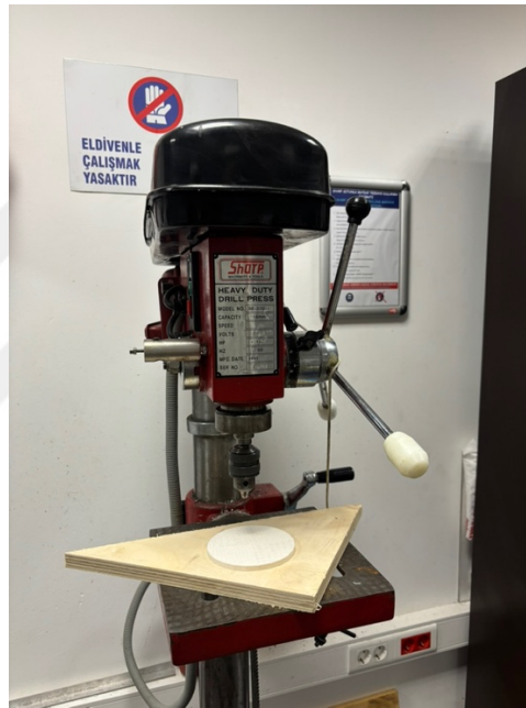
Figure 18. A heavy-duty drill press machine used to refine unprinted holes
