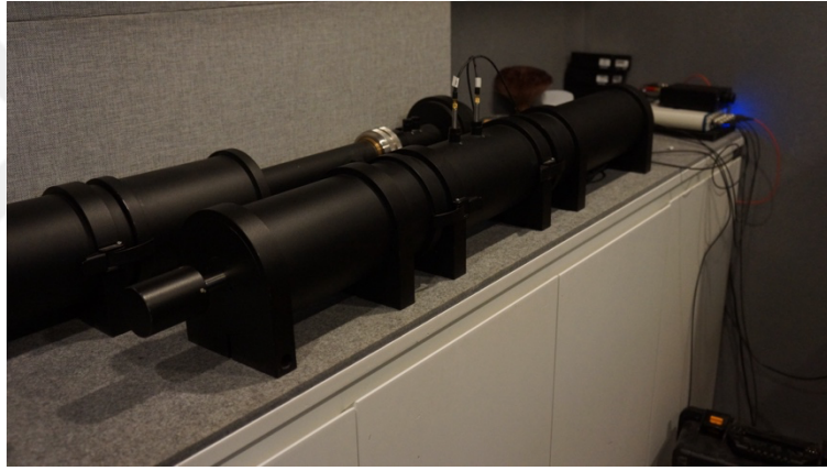
Figure 20. TestSense impedance tube at BLX Acoustic Research Lab (İzmir, Türkiye)
