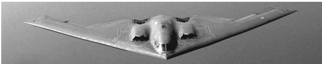
Figure 2.6 The B-2 stealth bomber aircraft, which is made of advanced composite materials. (Miracle & Donaldson, 2001)
