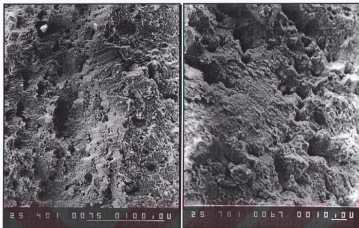
Figure 4.31 SEM fractographs of the typical fracture surface throughout the final fracture region showing dimple craters and inclusions
