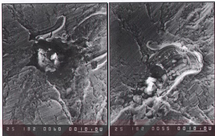
Figure 4.29 Fracture origin of Sample 8.500.20-6 and its mating part showing particle-matrix decohesion and deformation at a subsurface non-metallic inclusion
