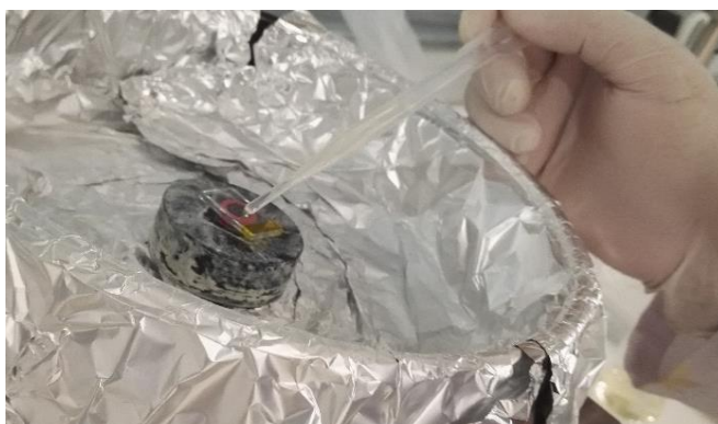
Figure 3.5 Spin Coating Process.
