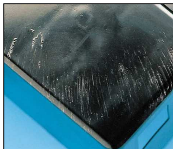
Figure 2.9 Charring streaks (Plasticportal, 2017)
