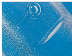
Figure 2.27 Stress cracking (Plasticportal, 2017)
