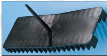
Figure 2.12 Deformation on demolding (Plasticportal, 2017)
