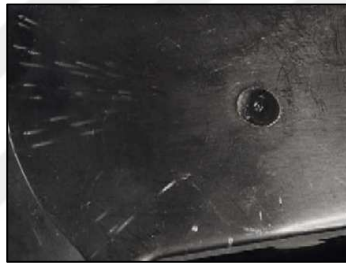
Figure 2.24 Moisture streaks (Plasticportal, 2017)
