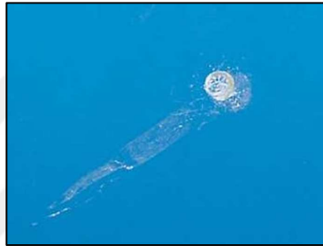
Figure 2.10 Cold slug (Plasticportal, 2017)
