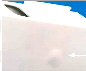
Figure 2.16 Entrapped air (Plasticportal, 2017)
