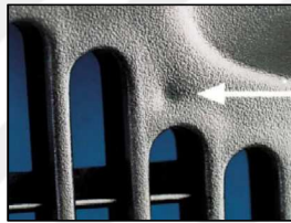
Figure 2.26 Sink marks (Plasticportal, 2017)
