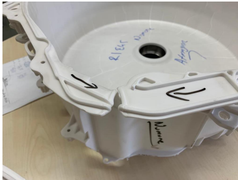
Figure 8: Short Shot Quality Failure in Production
