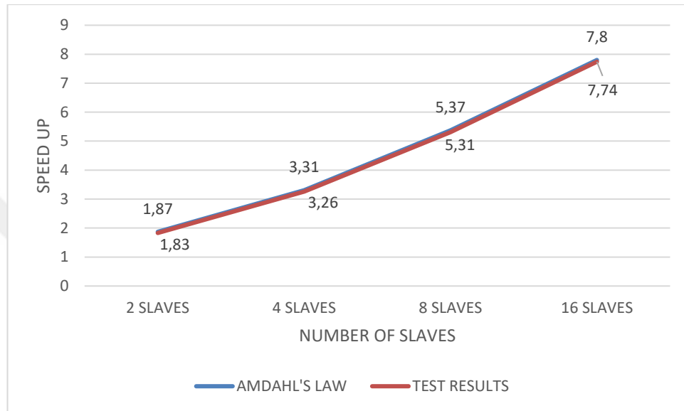
Figure 6.2 Comparison of speed up between Amdahl's law and matrix multiplication test results
