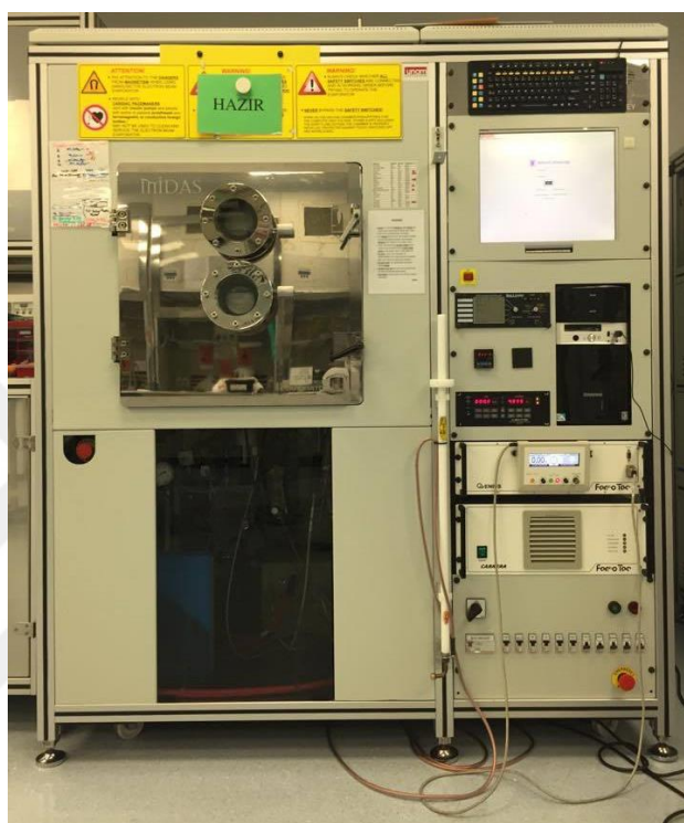
Figure 3.1 Vaksis MIDAS E-Beam evaporation system used for sample preparation.
