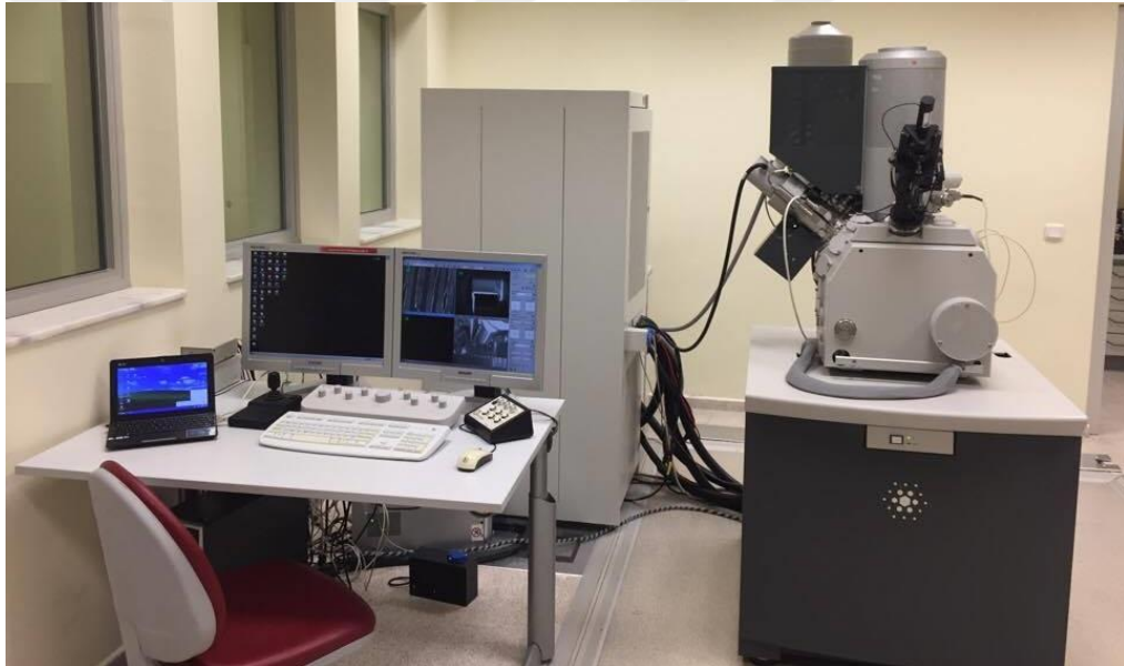
Figure 3.8 FEI Nova 600i Nanolab FIB device used to prepare cross-sectional TEM samples.
