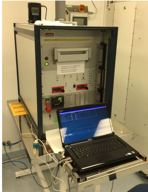
Figure 3.3 Rapid thermal annealing (RTA) system used to prepare samples.
