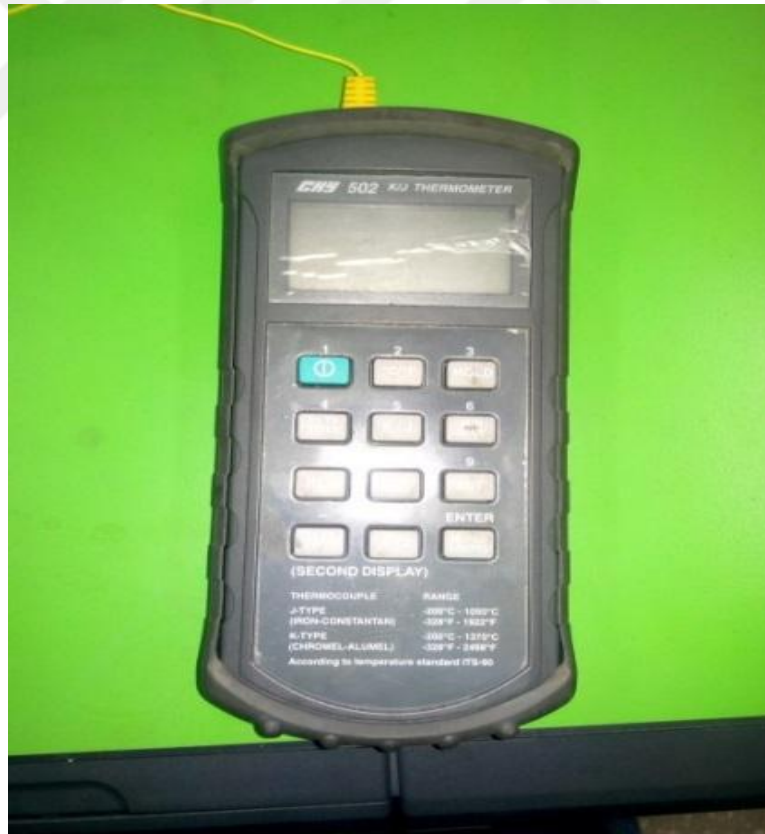
Şekil 5.4. Operating Instructions Model (W) 502 K/J termometre
