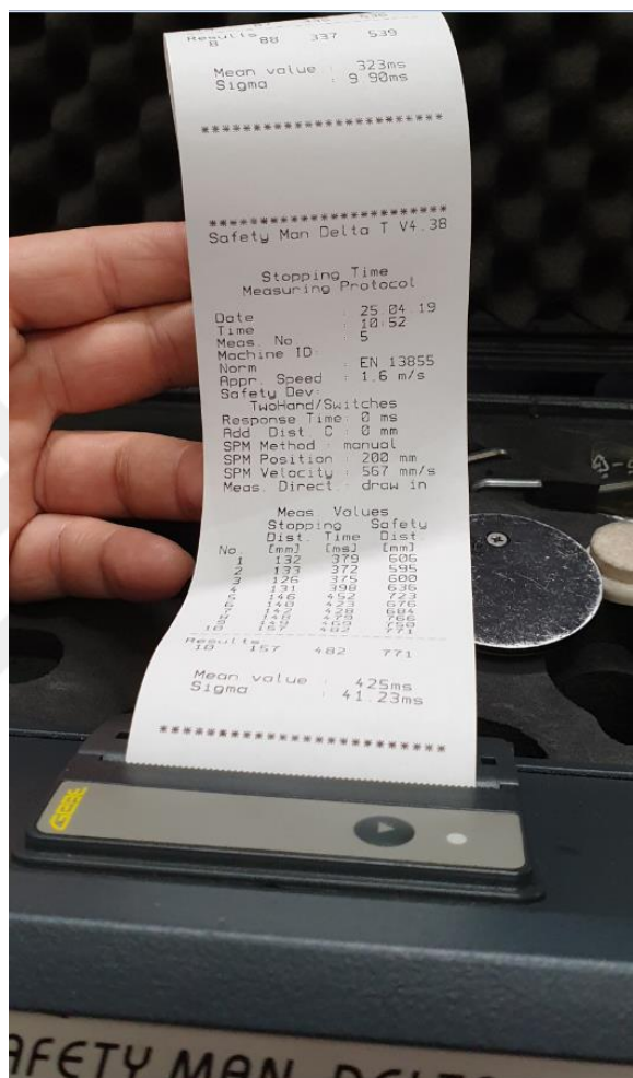
Figure 5.23 The safety distance of light curtain placement (Personal archive, 2019)
