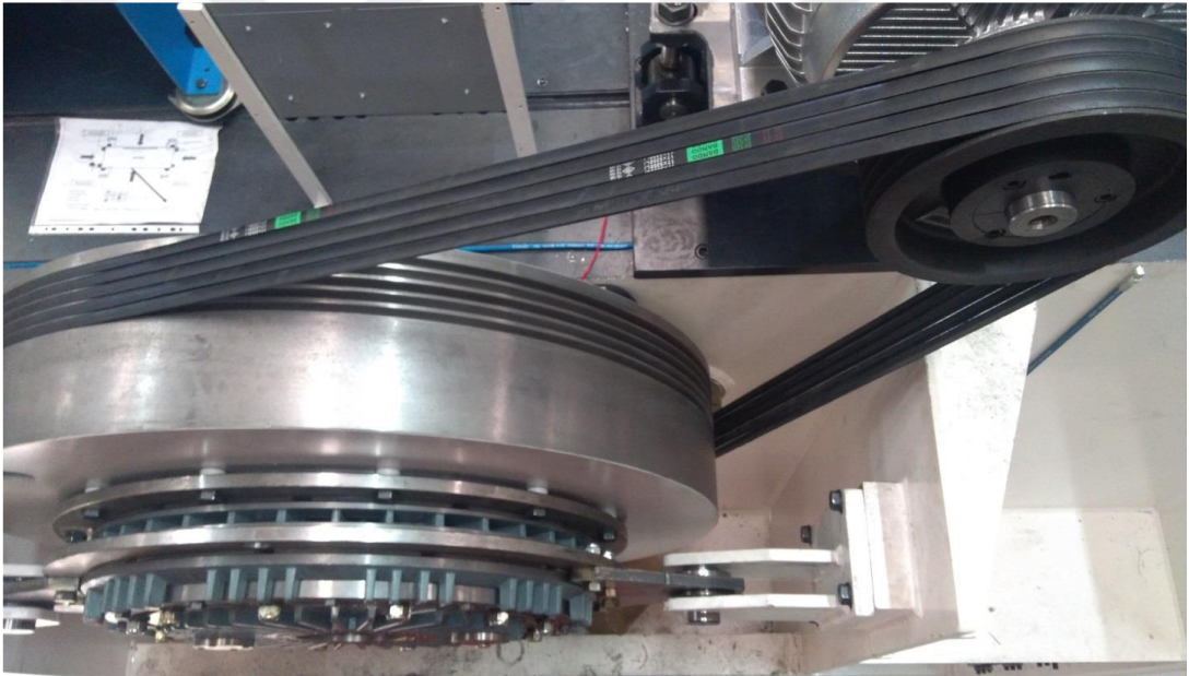
Figure 2.3 Flywheel which is connected to motor with belt (Dirinler Mak. San. ve Tic. A.Ş., 2019)
