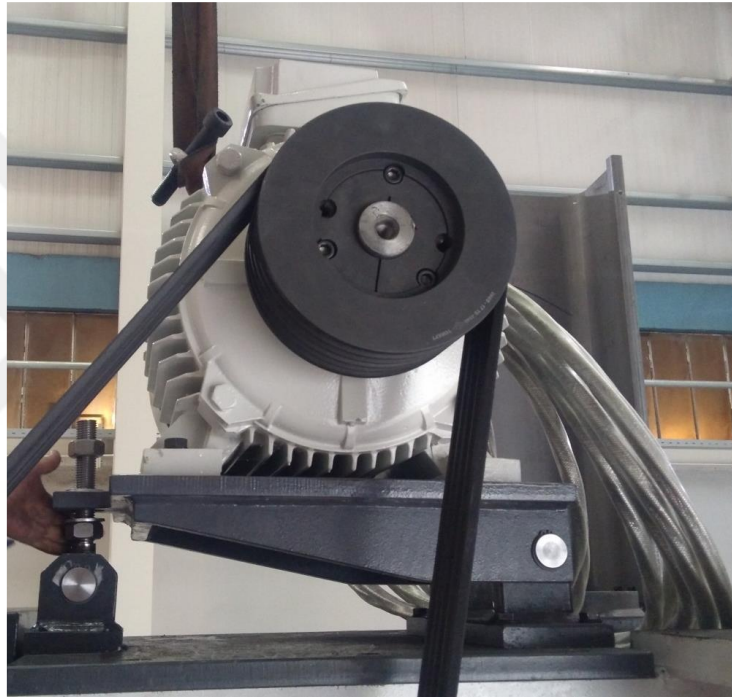
Figure 2.2 Electrical motor of press machine (Dirinler Mak. San. ve Tic. A.Ş., 2019)
