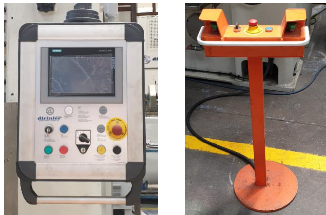
Figure 5.25 The emergency stop buttons that are placed are placed for double hand use and control panel (Personal archive, 2019)
