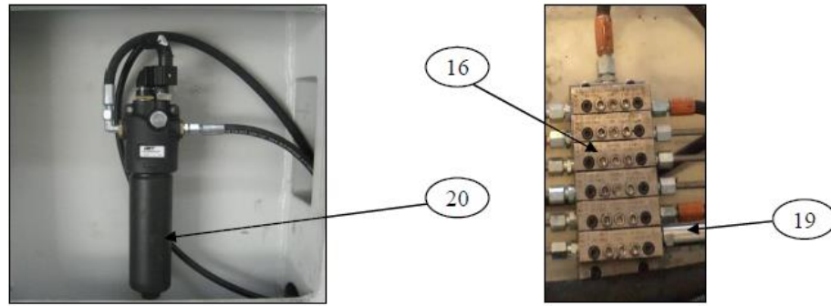
Figure 4.3 Oil dirtiness filter – oil distribution System (Dirinler Mak. San. ve Tic. A.Ş., 2019)
