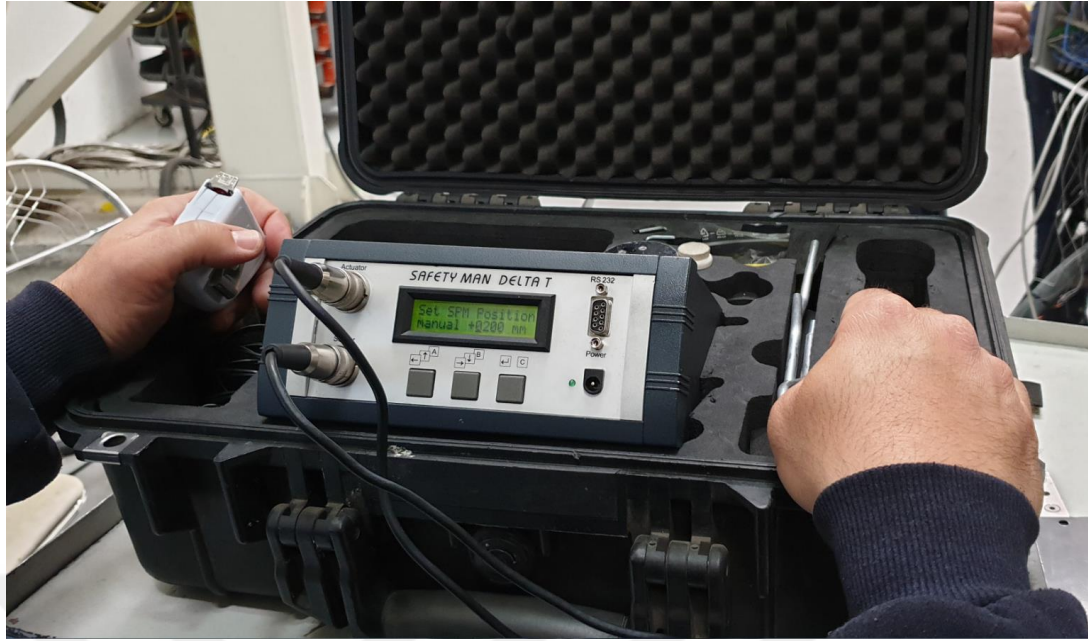
Figure 5.21 The distance calculator device of light curtain parameters (Personal archive, 2019)
