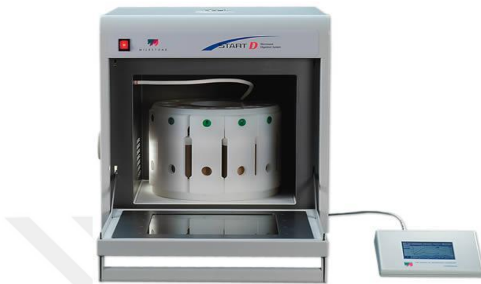
Figure 3.6. A Milestone Start D (Sorisole, Italy) microwave digestion system
