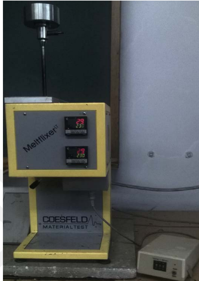
Figure 3.8. Photograph of melt flow rate device used in this study.
