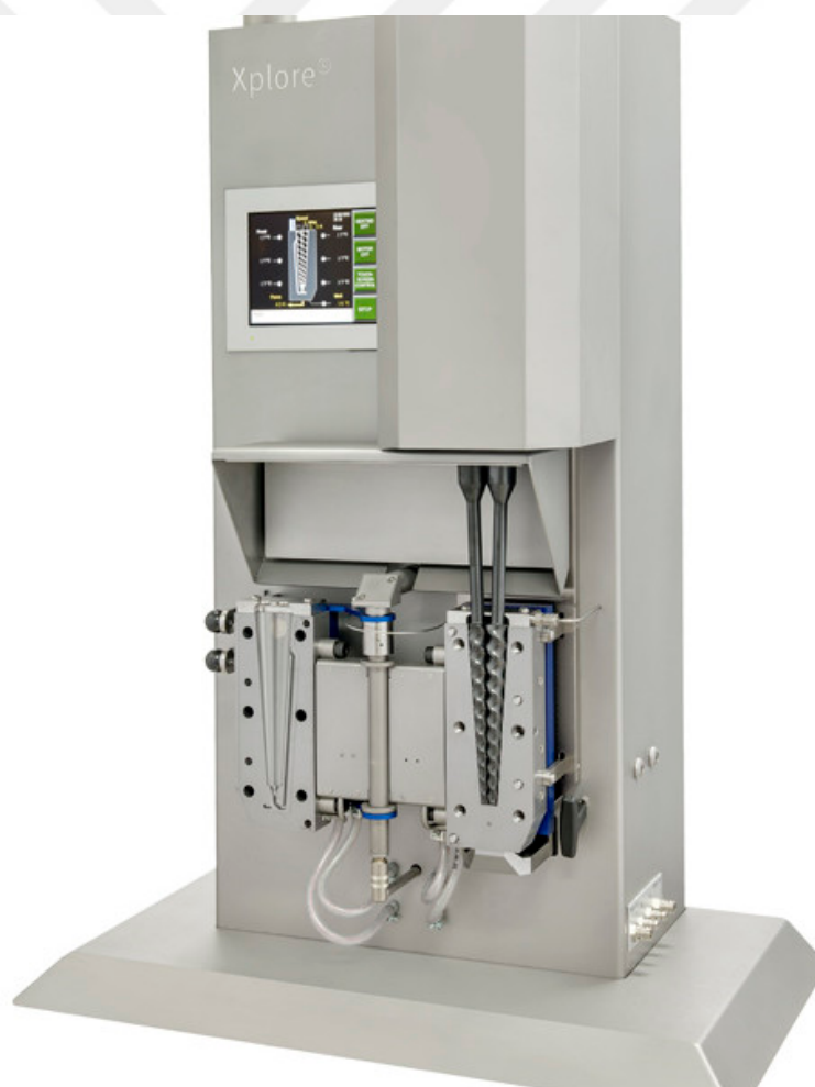
Figure 3.2. The lab-scale micro-compounder used in this study.
