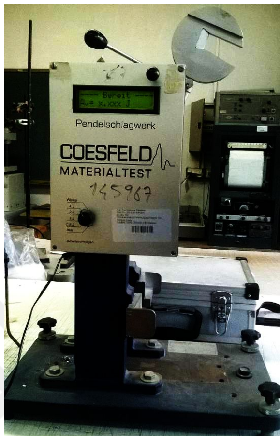
Figure 3.7. Photograph of impact tester device used in this study.
