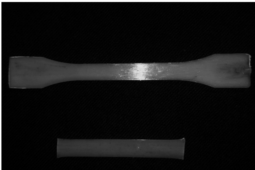
Figure 3.4. Photograph of prepared test specimens by injection molding.
