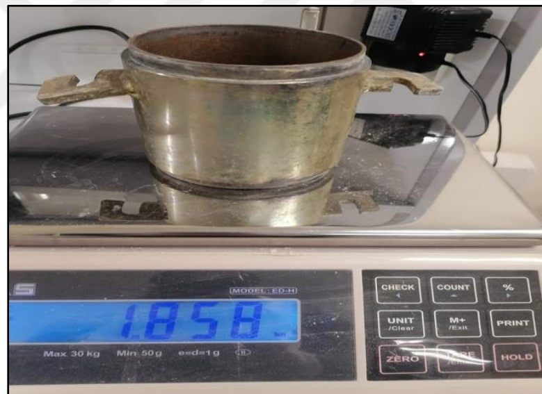
Figure 3.18. Taking weight the empty mold
