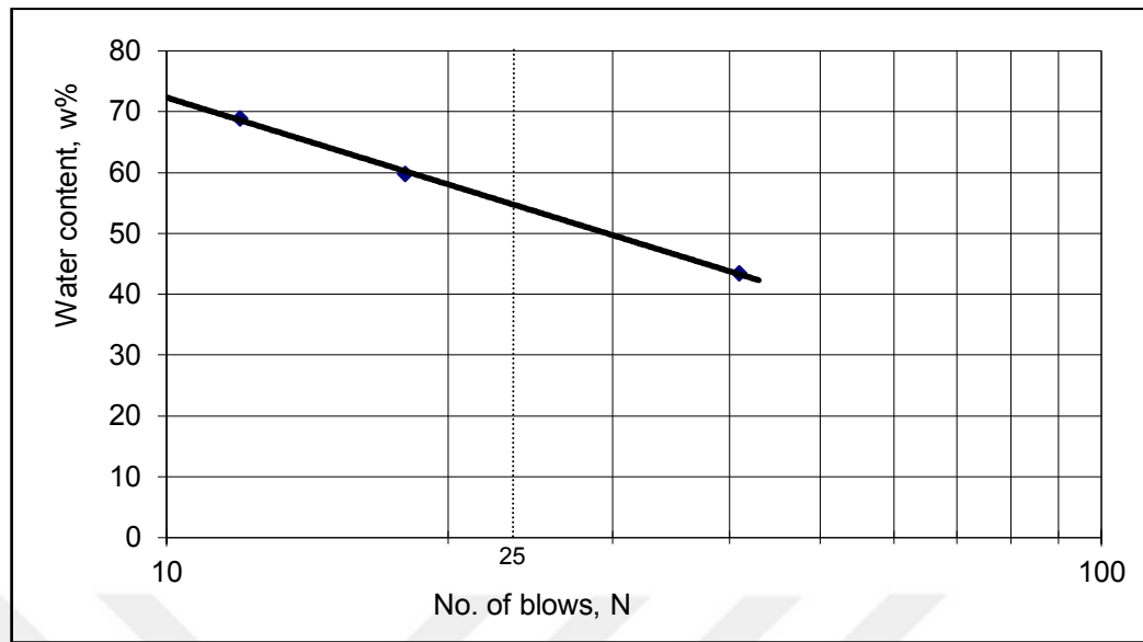
Figure 4.1. The liquid limits graph of the sand-bentonite mixture without addition
