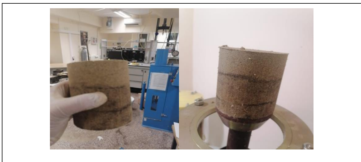
Figure 3.20. The sample after the compaction processes
