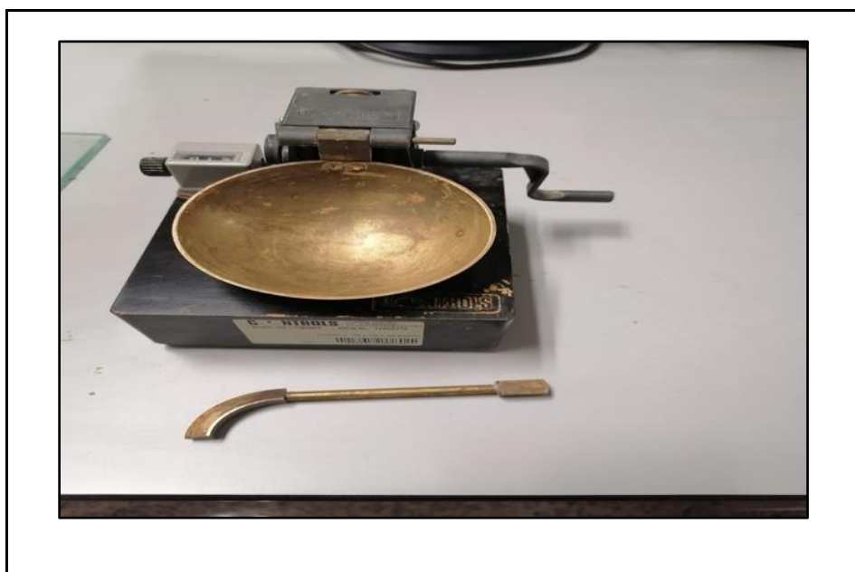
Figure 3.12. Liquid limit machine and grooving tool (Casagrande cup)
