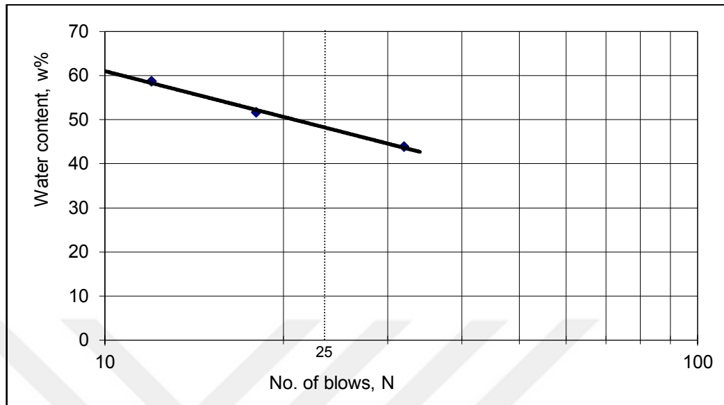
Figure 4.17. LL graph of the sand-bentonite mixture with 0.2 % tire chips addition
