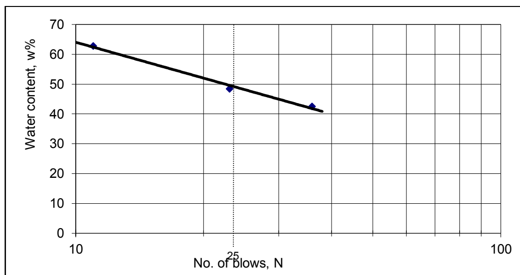
Figure 4.16. LL graph of the sand-bentonite mixture with 0.1 % tire chips addition
