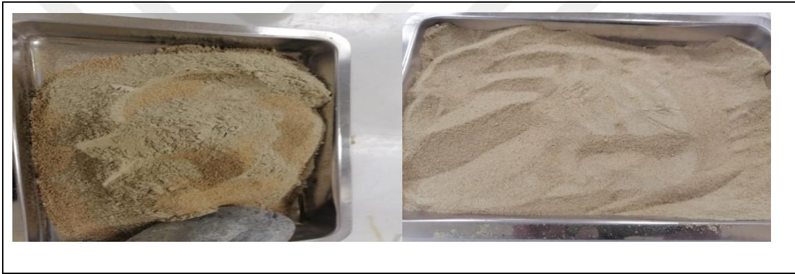
Figure 3.13. Mixing the sand-bentonite in homogeneity
