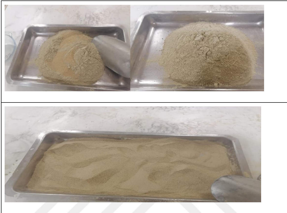
Figure 3.10. Mixing the dry sand with bentonite
