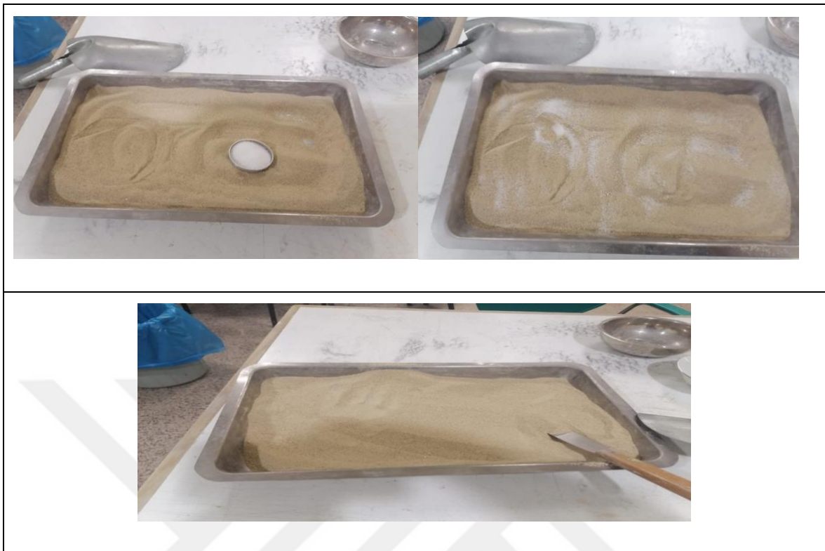
Figure 3.11. Mixing the sand-bentonite mixture with polyacrylamide homogenously
