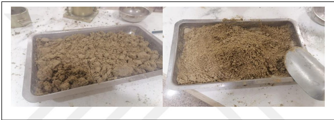
Figure 3.21. Crushing the remaining sample and remixing it by addition water
