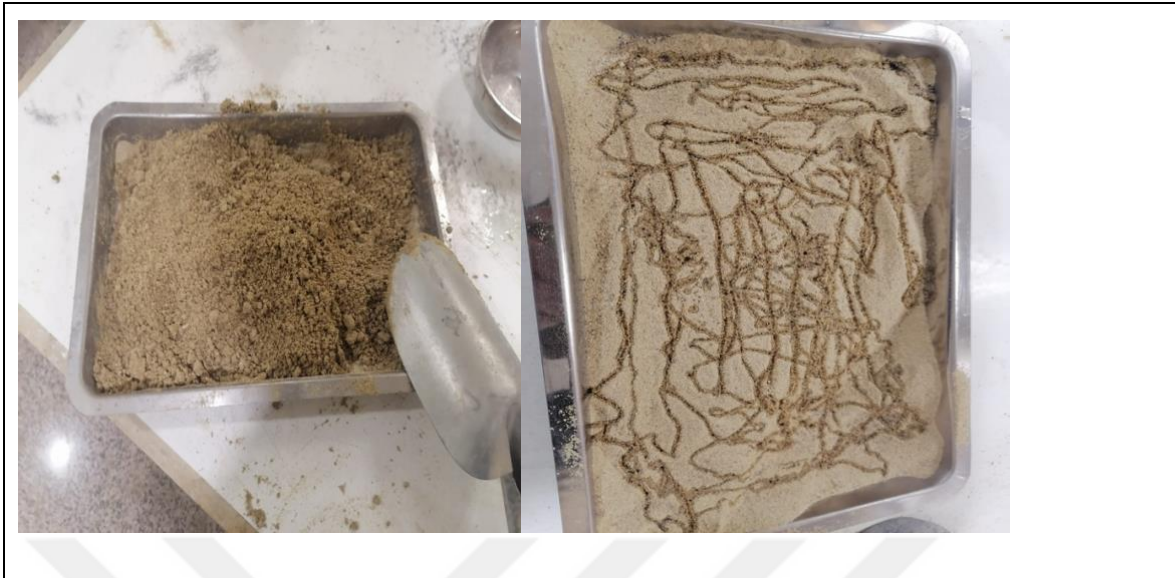
Figure 3.17. Mixing the water with sand bentonite mixture
