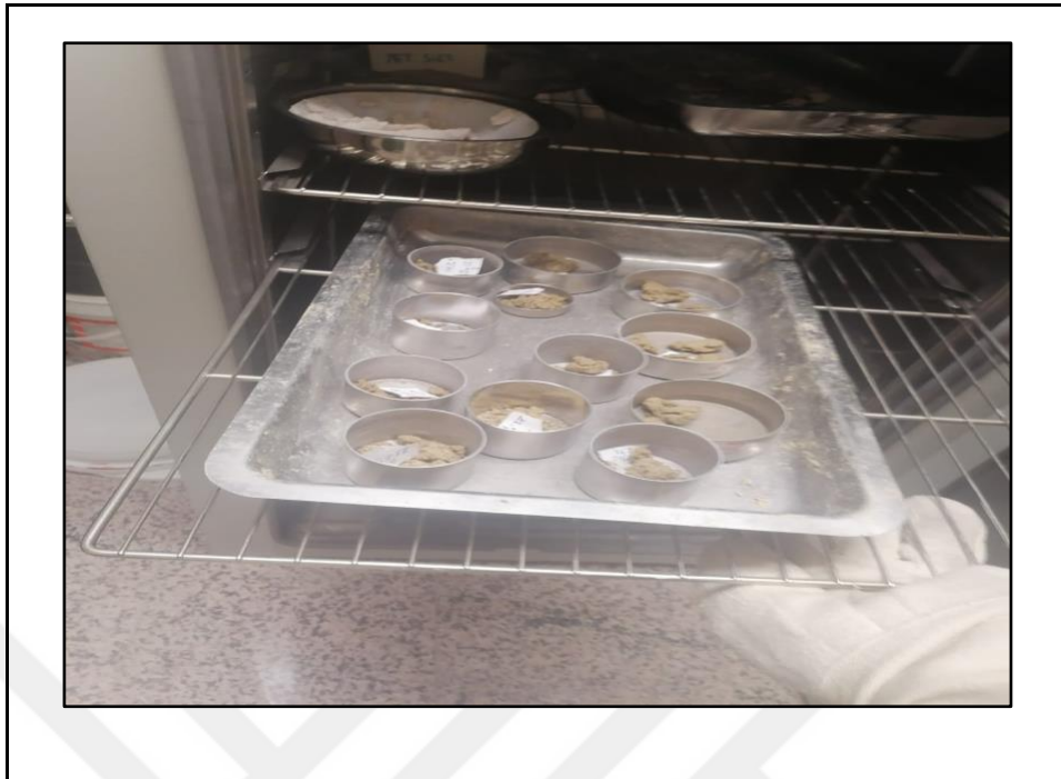
Figure 3.15. Water content determination by putting the samples in the oven
