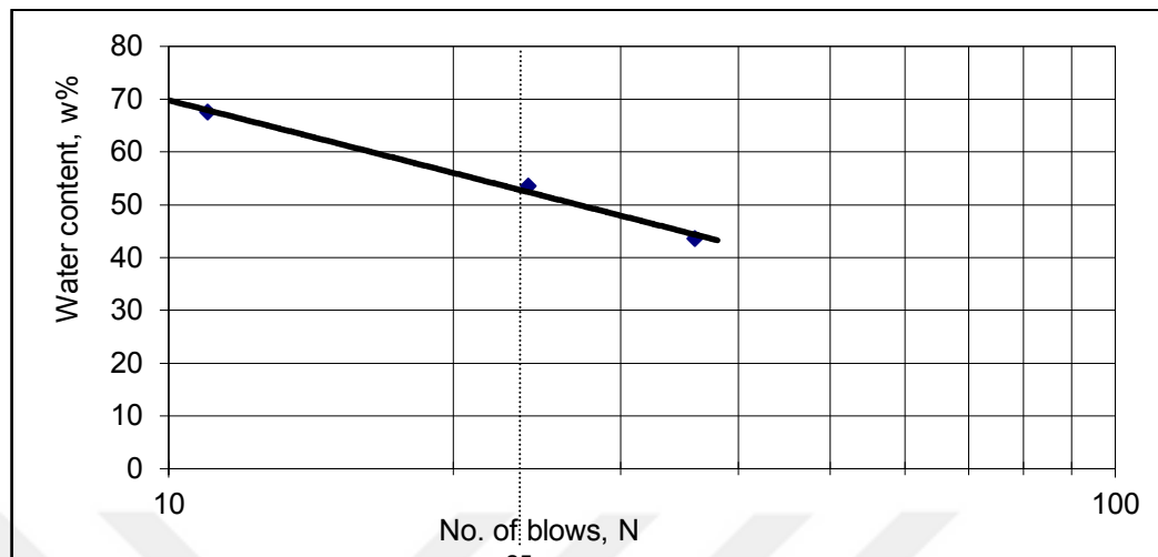
Figure 4.5. LL Graph of the sand-bentonite mixture with 0.5% cationic addition
