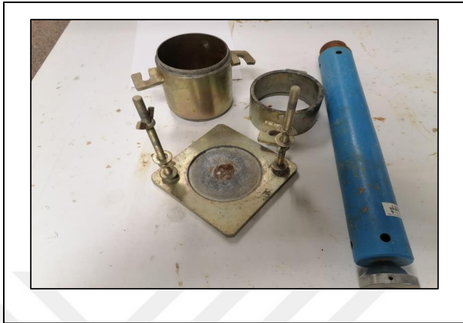
Figure 3.16.' Proctor test equipment mold and hammer
