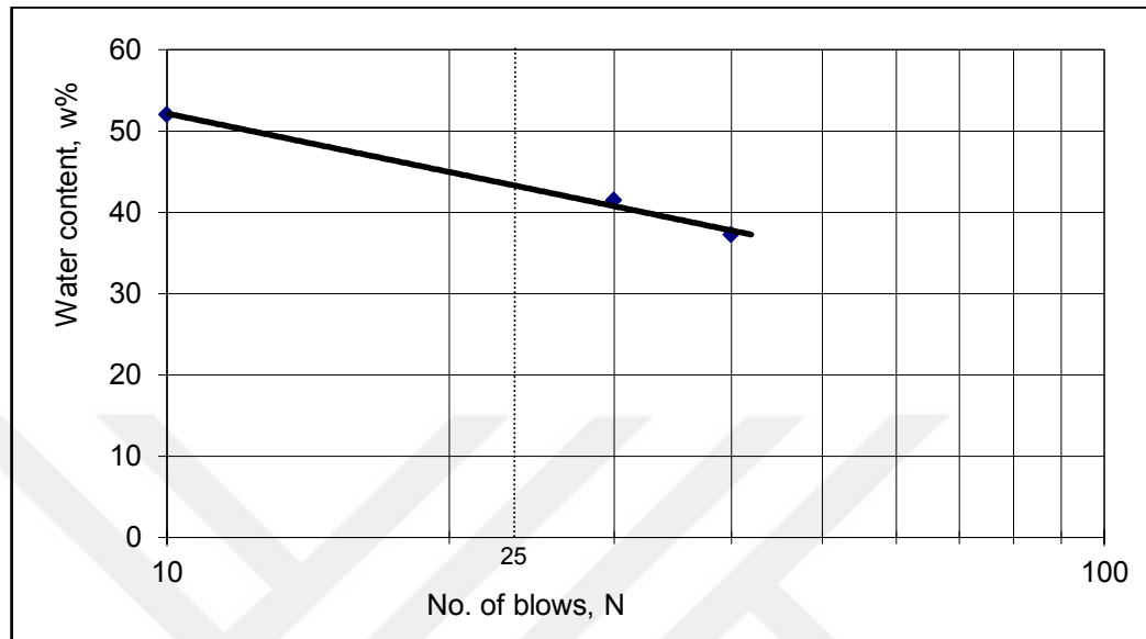
Figure 4.7. LL Graph of the sand-bentonite mixture with 2 % cationic addition
