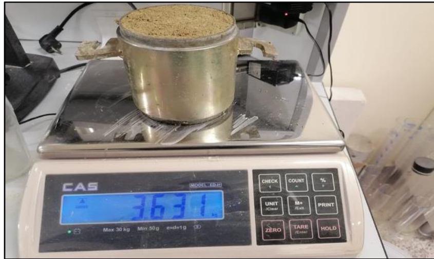
Figure 3.19. Taking weight the wet sample with the mold
