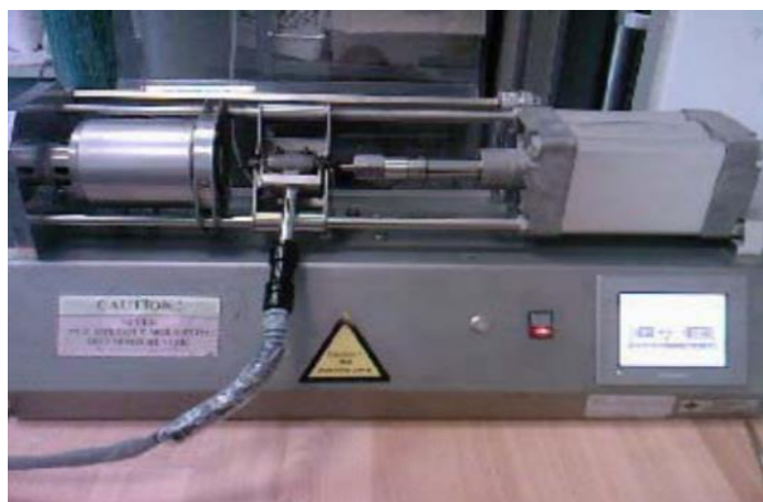
Figure 3.4. A photograph of the DSM Xplore, laboratory-scale micro injection molding.
