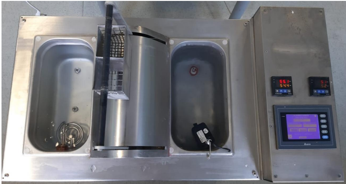
Figure 3.19. Thermocycling device. (Salubris Technica, Dentester, Turkey)
