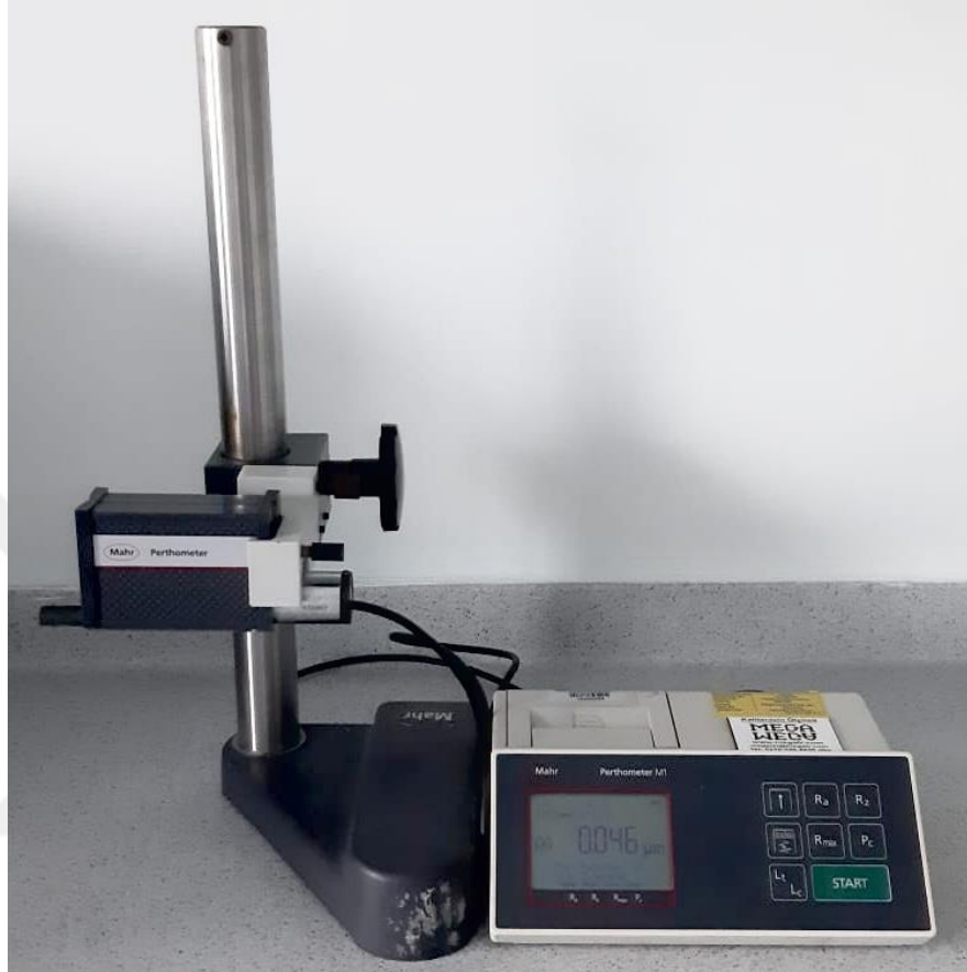
Figure 3.4. Illustration of profilometer. (Perthometer M1, MAHR, Germany)
