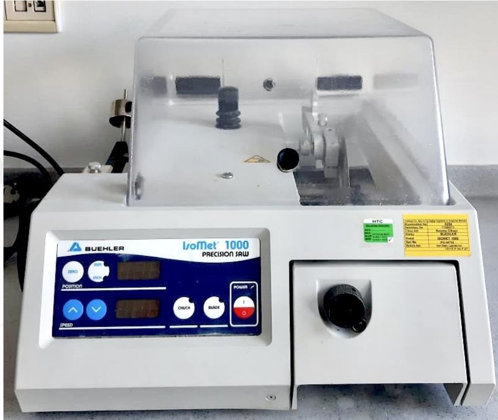
Figure 3.1. Illustration of device for PEEK specimen dissection. (BUEHLER, ISOMET 1000, Germany)
