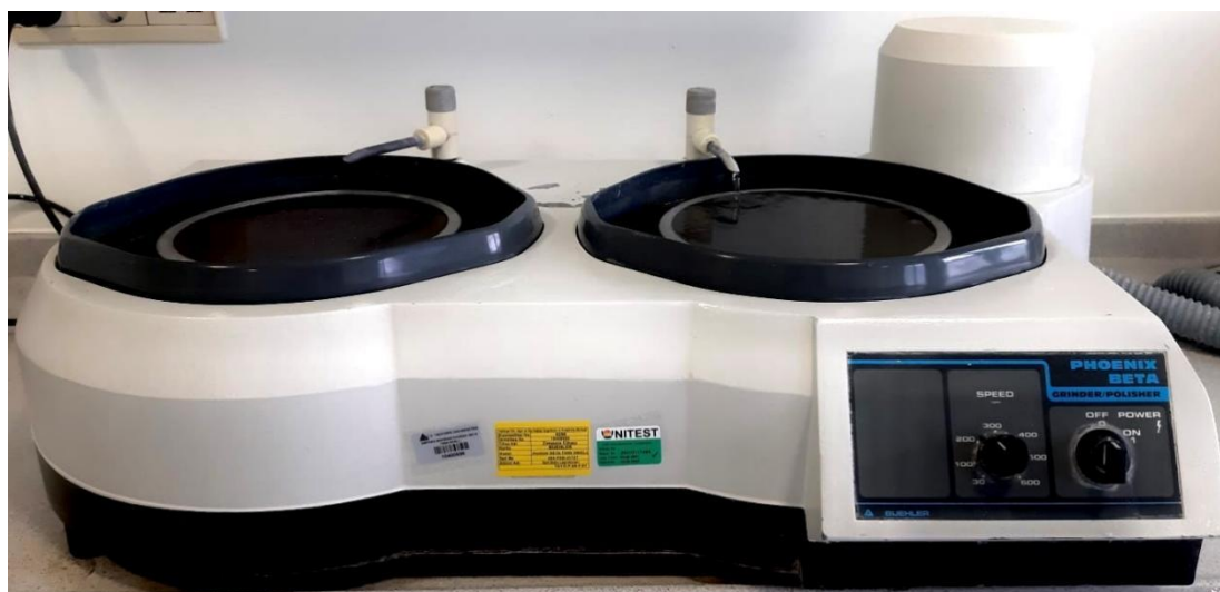
Figure 3.3. Illustration of polishing device. (Phoenix Beta Twin Whell, Buehler, Germany)
