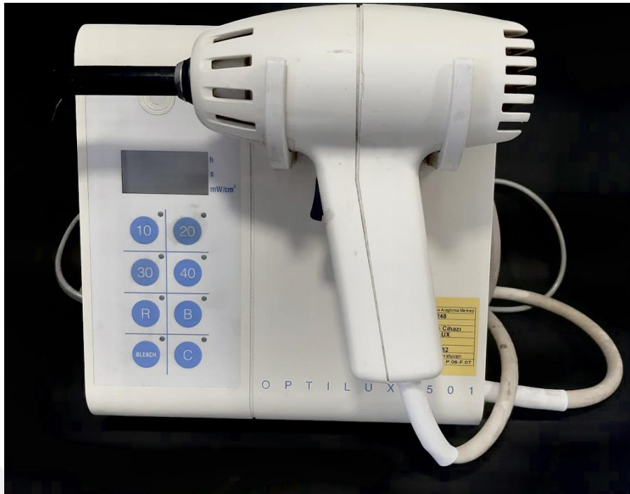
Figure 3.15. Illustration of light curing machine (OPTILUX 501).
