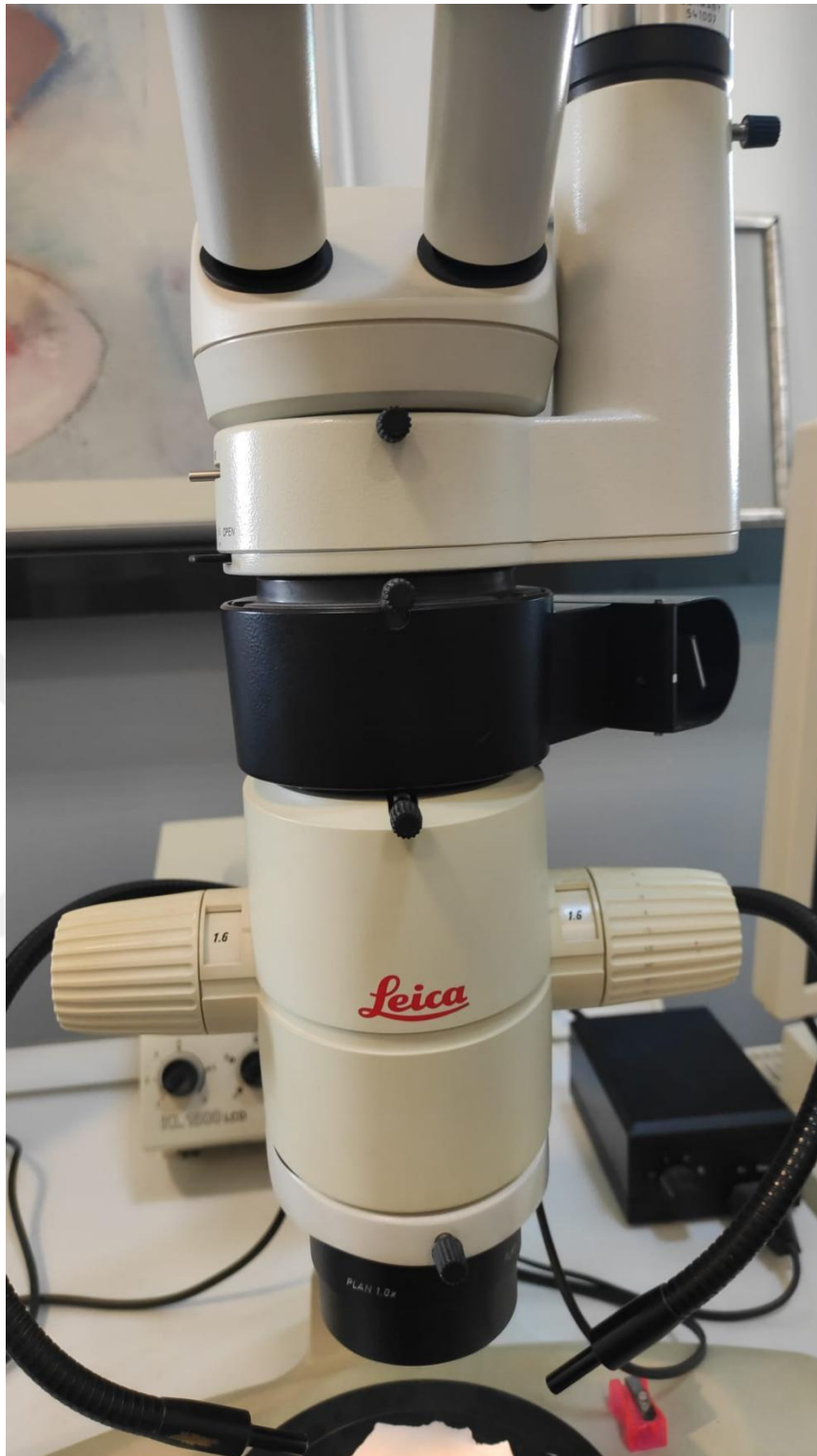
Figure 3.23. Illustration of stereomicroscope. (Leica, MZ10F, Germany)
