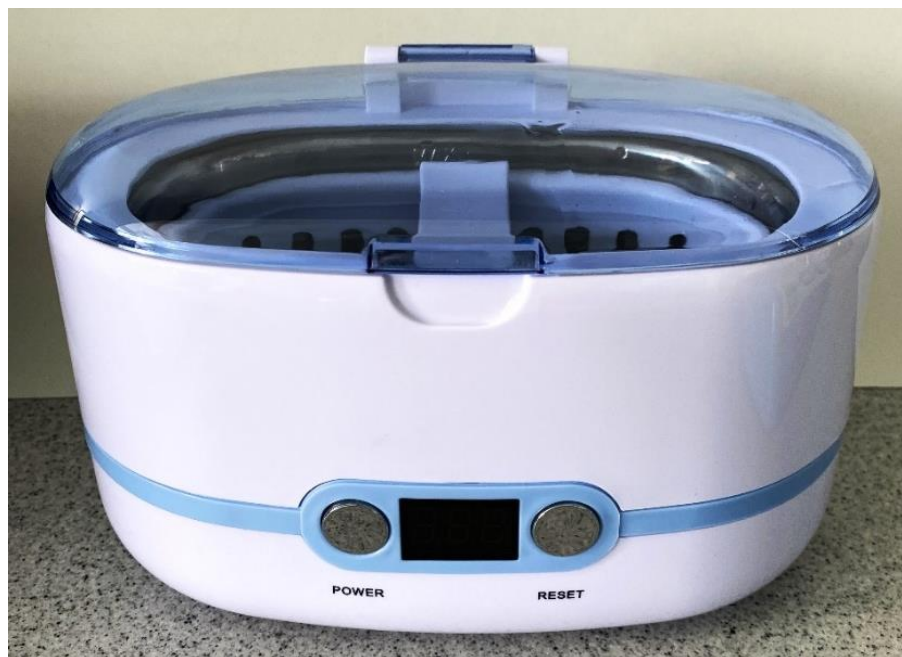
Figure 3.9. Ultrasonic bath for cleaning the samples. (Tchibo GmbH, Germany)
