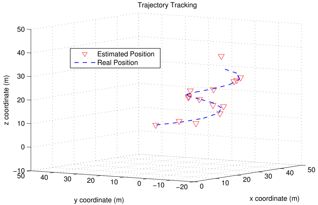
Figure 6.4 The trajectory tracking with positioning system designed with 3 element antenna array system
