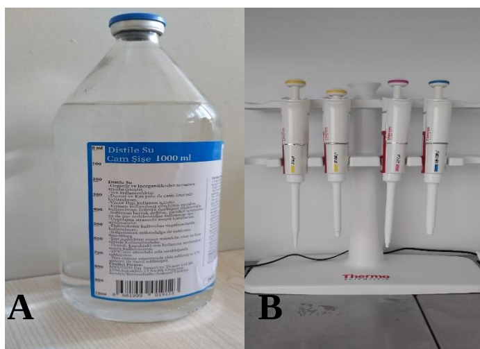
Figure 3.5. A- Distilled water used for dissolving substances like agmatine B- Different sizes of pipettes that are used in the calculation of fluid size in ml and \mu\text{l}
