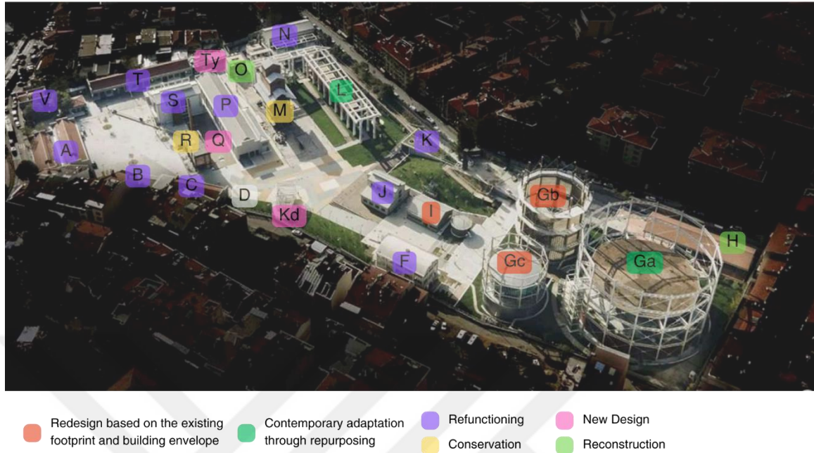
Figure 3.14 Schematic plan of Hasanpaşa Gasworks generated by the author, incorporating building codes pertinent to conservation and design principles (Source: Tanyeli & Salman, 2021)
