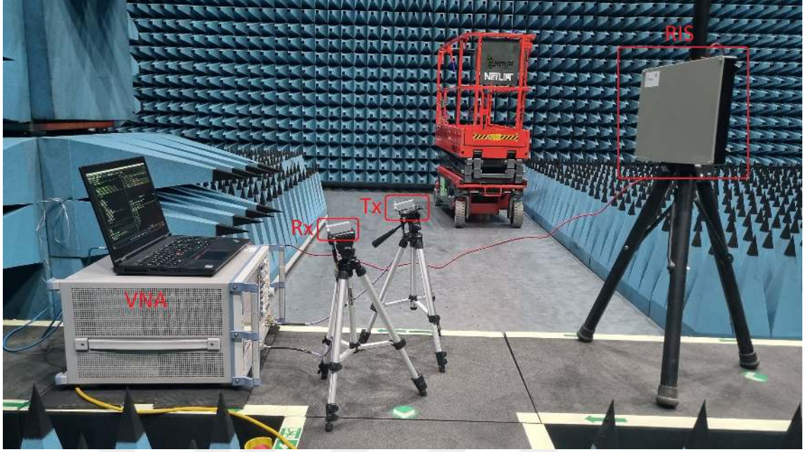
Figure 6.2: The measurement setup constructed to validate the performance of the mmWave RIS in an anechoic chamber.
