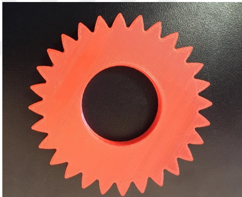
Figure 3.16 The 3D printed model of the prototype gear
