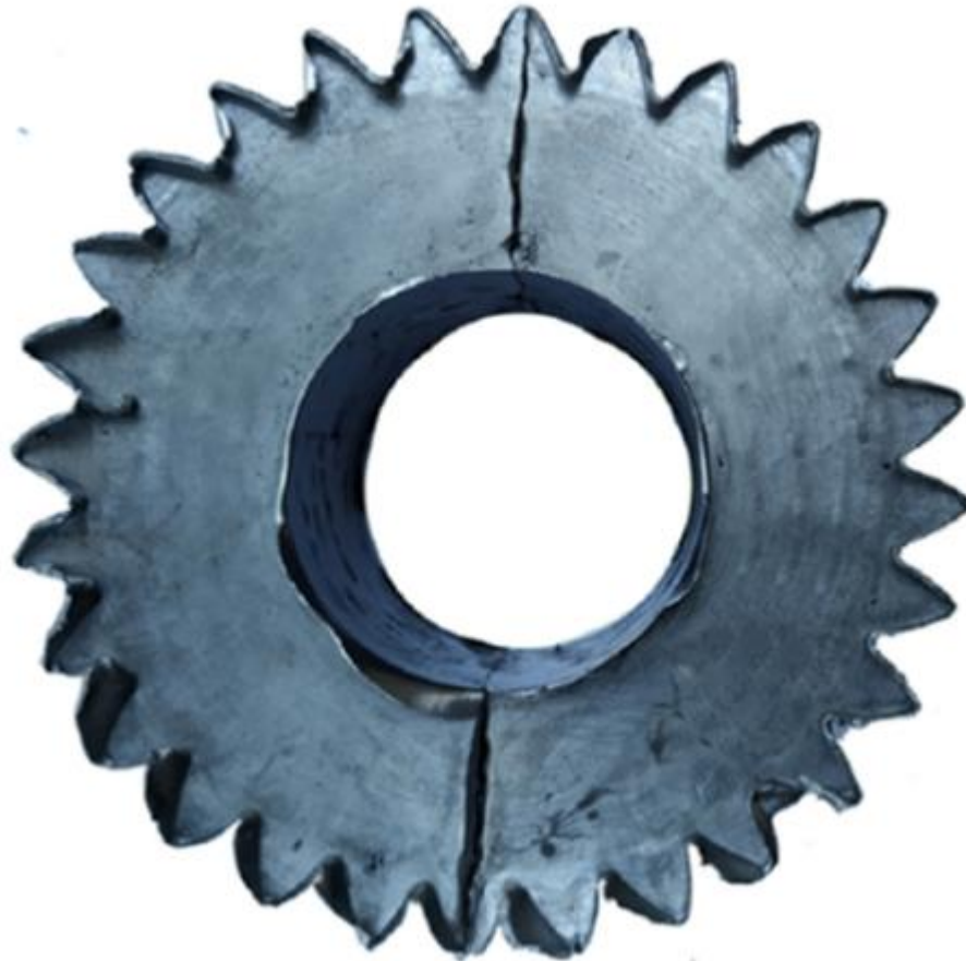
Figure 8.8 Asymmetric spur gear resulting from forging
