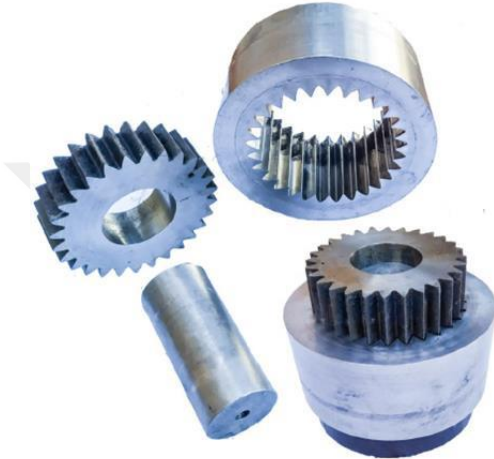
Figure 7.4 The components of the forging die set
