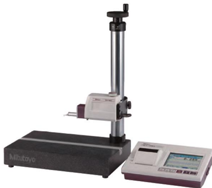
Figure 7.8 Mitutoyo SJ 401 Surface roughness tester
