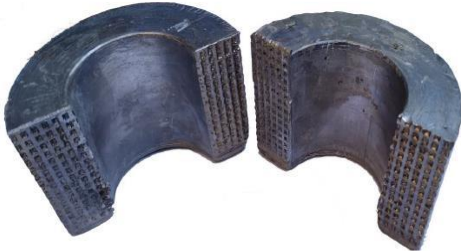
Figure 7.1 Two halves preform with grids
