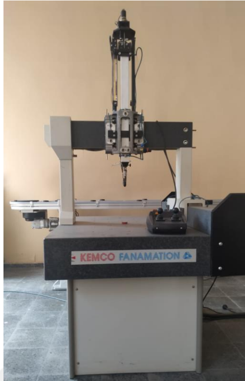
Figure 7.7 The Kemco 3D Coordinate Measuring Machine (CMM)
