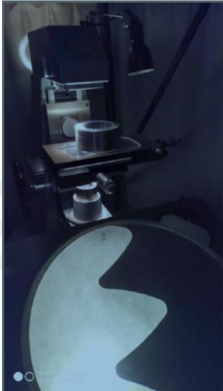
Figure 7.6 Magnified tooth profile by using Leitz Wetzlar optical profilometer
