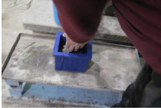
Figure 4.9: Compaction of specimens by table vibrator.
