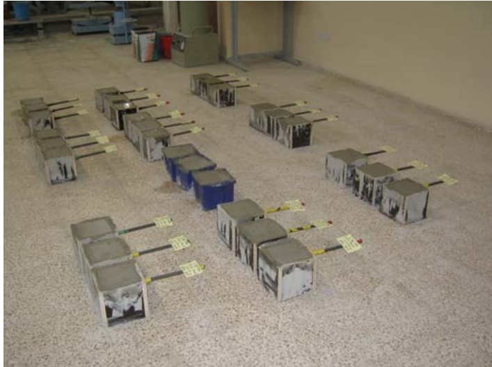
Figure 4.34: First group of concrete specimens ( w/c= 0.75 ) after compacting.
