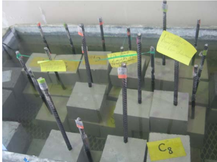
Figure 4.25: 28 days water curing of first trial concrete specimens.
