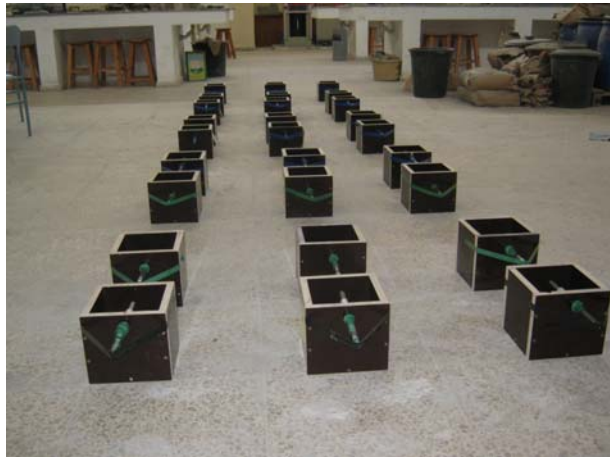
Figure 4.52: Set up of concrete specimens ( w/c= 0.40 ) before casting concrete.
