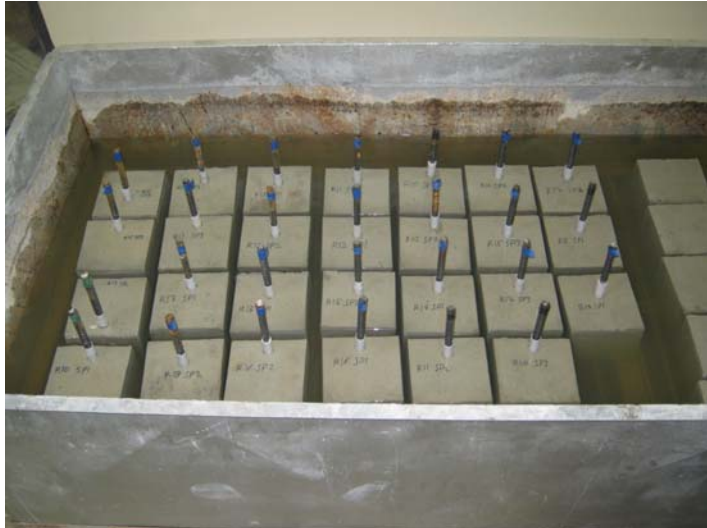
Figure 4.37: 28 days water curing of concrete specimens with a water/cement ratio of 0.40.
