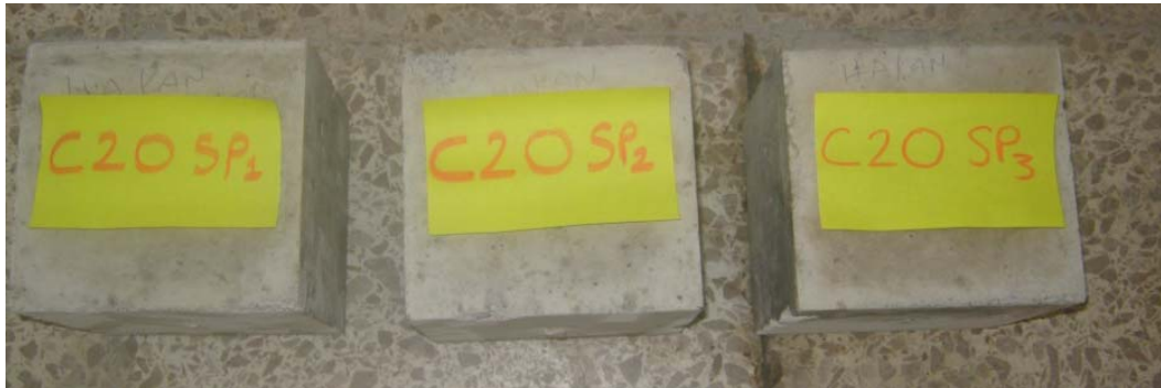
Figure 4.6: Trial mix design with a water/cement ratio of 0.75.
