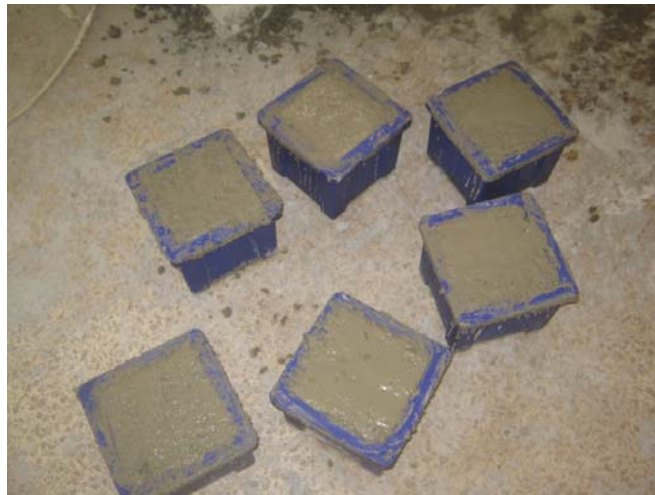
Figure 4.7: Trial mix design with a water/cement ratio of 0.40.
