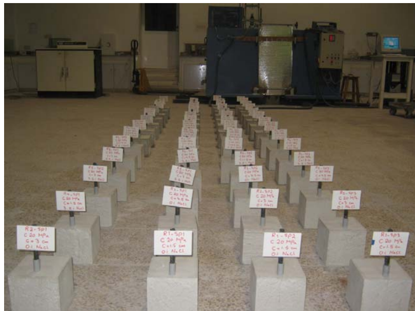
Figure 4.38: 28 days after water curing of concrete specimens with water/cement ratios of 0.75 and 0.40.
