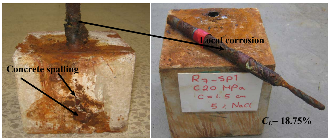
Figure 5.5: Spalling of concrete with highest amount of corrosion level.
