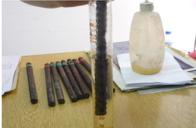
Figure 5.7: Application of Archimedes's principle due to occurred local corrosion.
