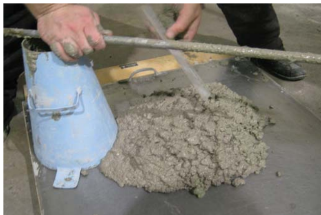
Figure 4.8: Slump test of designed concrete specimens.
