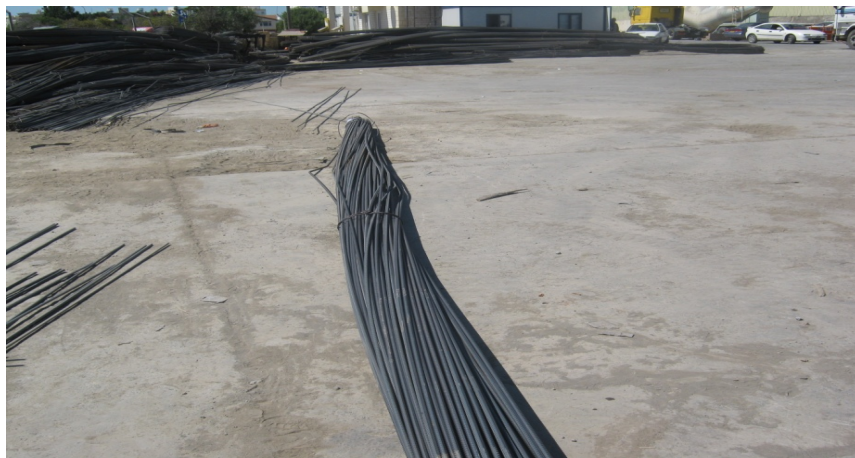
Figure 4.3: Used non-corroded reinforcement bars.
