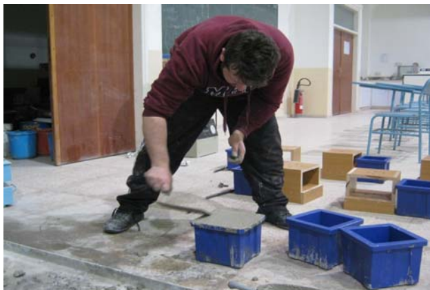
Figure 4.10: Smoothing the surface of specimens.
