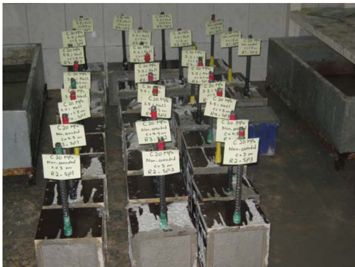
Figure 4.35: Curing of concrete specimens with a water/cement ratio of 0.75
