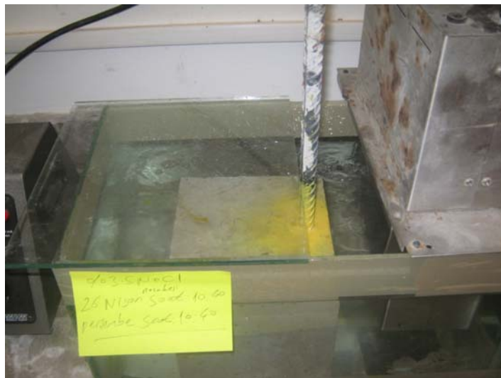
Figure 4.28: Painted reinforcement bar to prevent local corrosion.
