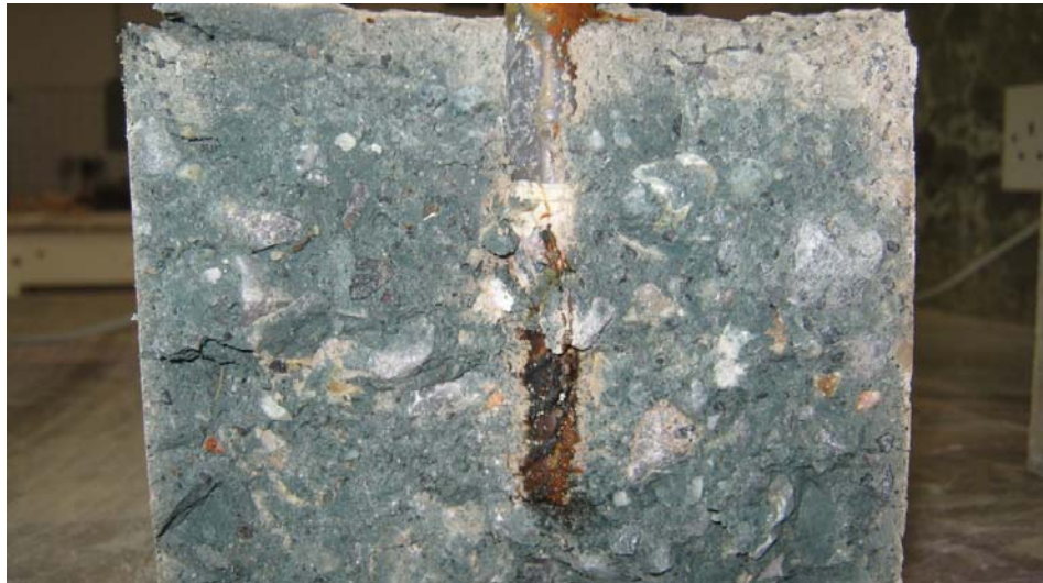
Figure 4.42: Broken concrete specimen after using PVC pipes.
