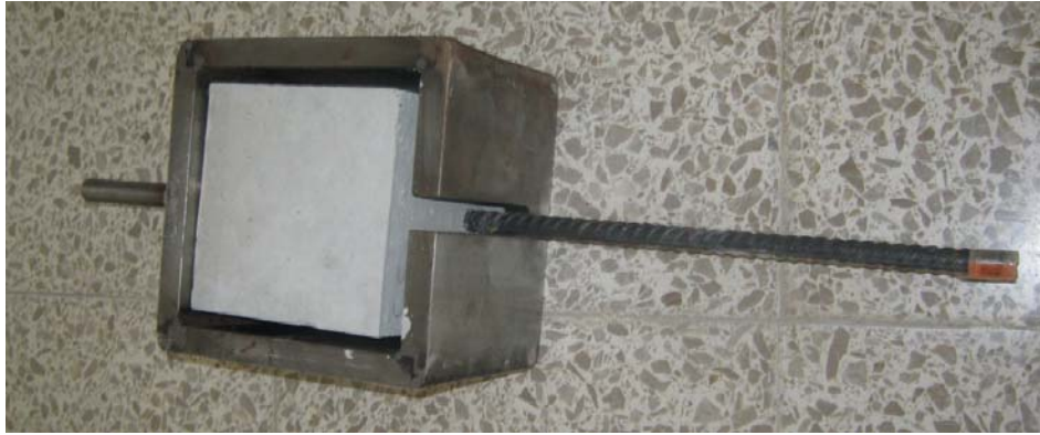
Figure 4.17: Designed apparatus for pullout test
