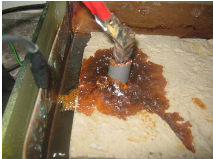
Figure 4.29: Prevention of local corrosion by PVC pipes.
