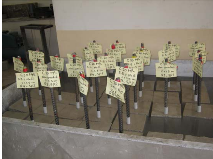
Figure 4.50: 28 days water curing of concrete specimens with a water/cement ratio of 0.75.
