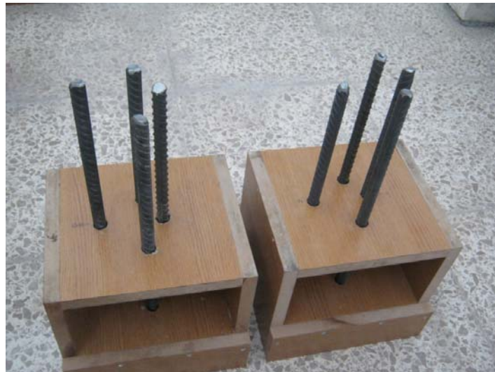
Figure 4.21: Alignment of the reinforcement bars for different concrete cover depths.
