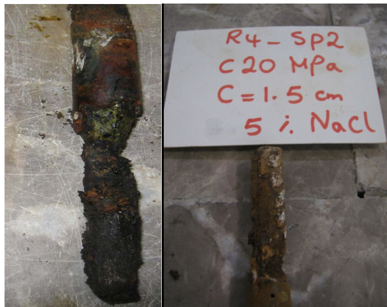
Figure 5.22: Damaged lugs of the reinforcement bars.
