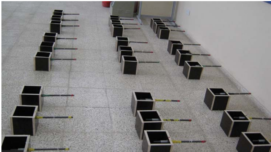
Figure 4.33: Set up of first group ( w/c= 0.40 ) of 27 specimens before casting concrete.
