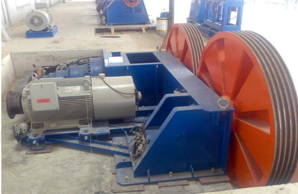
Figure 4.4. Capstan blocks (Kemtech, 2014)
