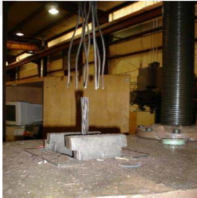
Figure 4.6. PC Strand specimen (ANONYMOUS)
