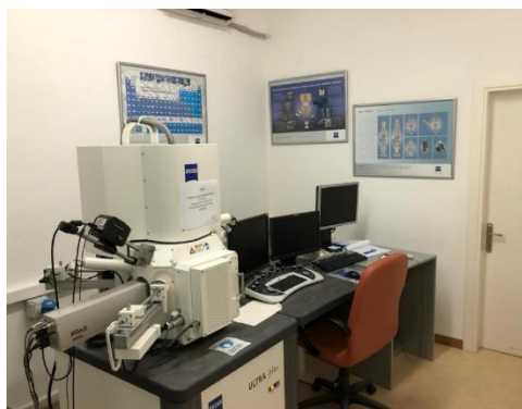
Image 5.8 Zeiss Ultra Plus FE-SEM and EDAX Pegasus system
