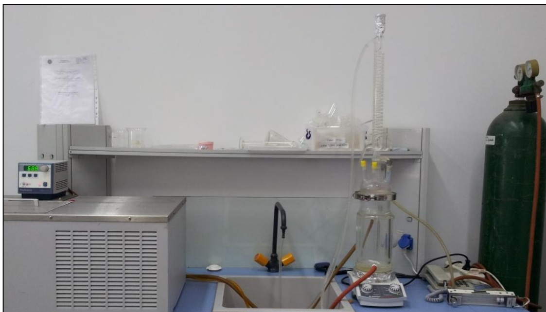
Figure 4.1 The glass reactor system used for MSN synthesis and polymer coating
