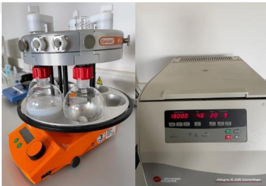
Figure 3.1. Polymerization reactor and high-speed centrifuge used for AgII-MIP and NIP nanoparticle synthesis.
