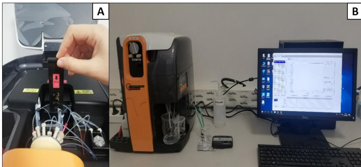
Figure 4.8. A) Placing the SPR chip into the device B) Taking sensorgrams from chips using an SPR device.
