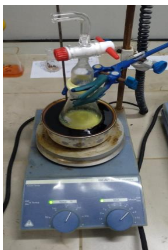
Figure 4.1. The mixture of polymer in oil bath on hot plate magnetic stirrers
