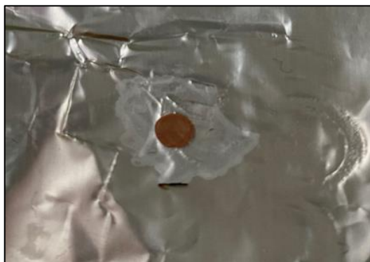
Figure 3.1. The grid preparation for the TEM characterization with MCM-41 nanoparticles
