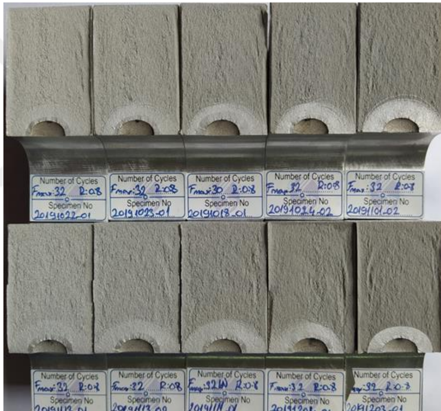
Figure 4.35. Fracture surfaces from 3-D fatigue crack growth tests under R= 0.8 constant amplitude
