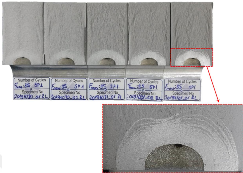
Figure 4.43. Tops views of 3-D crack fronts and a close-up view of FCG region
