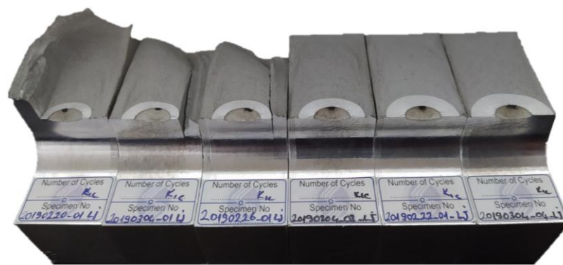
Figure 4.28. Lee James specimen used in fracture toughness tests
