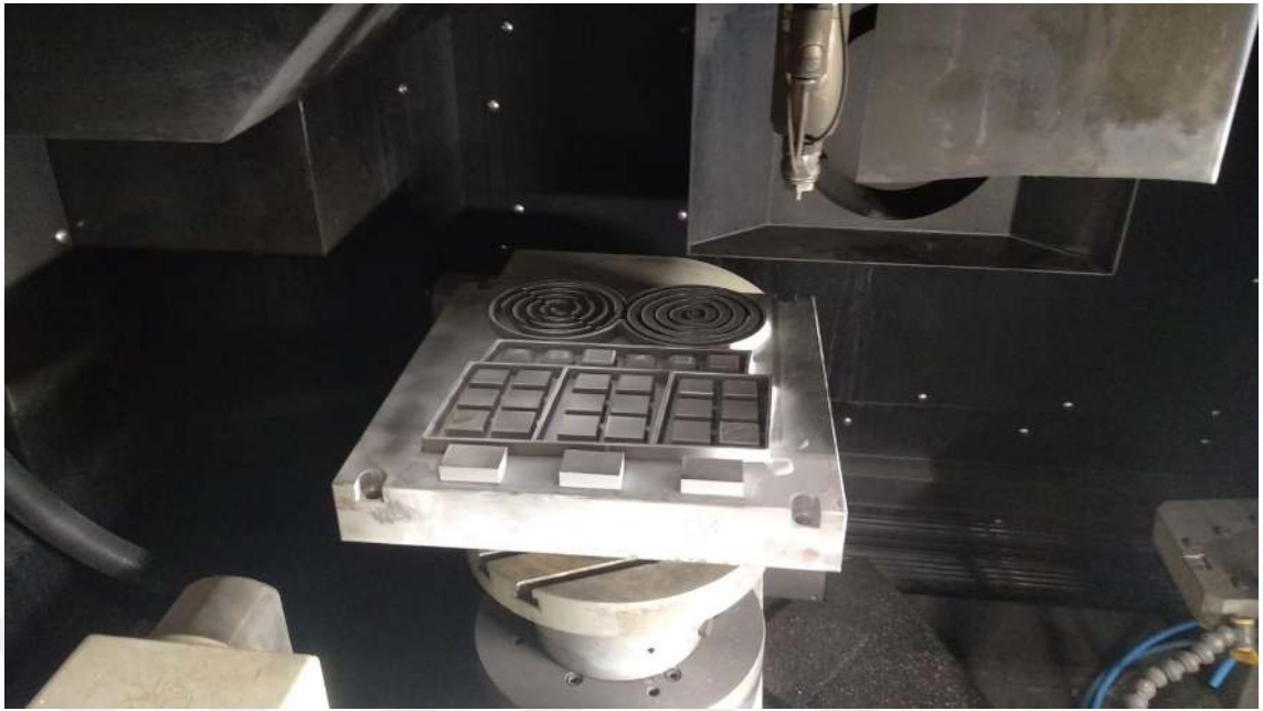
Figure 4.14 Synova MicroJet Laser system and test part
