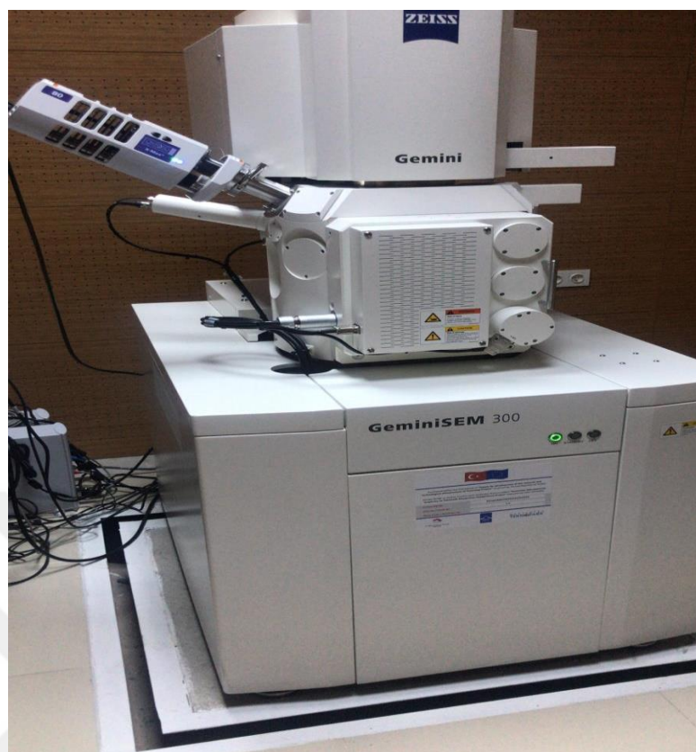
Figure 3.9 FE-SEM, GeminiSEM 300 (ZEISS, USA)
