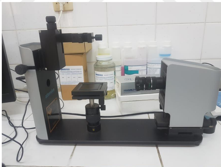
Figure 3.2 Surface tension meter instrument
