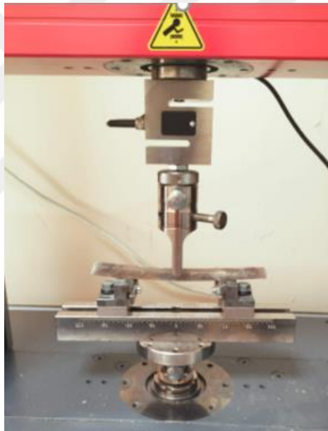
Figure 3.7. Flexural strength testing
