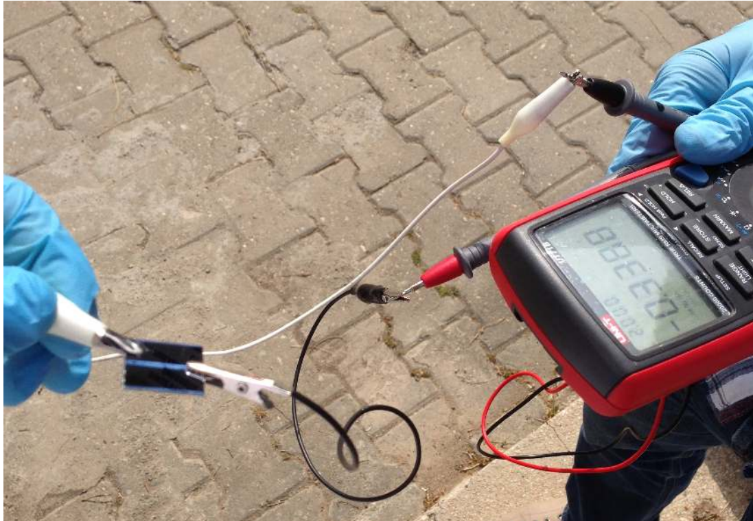
Figure 4.23 Single solar cell test under sunlight with multimeter
