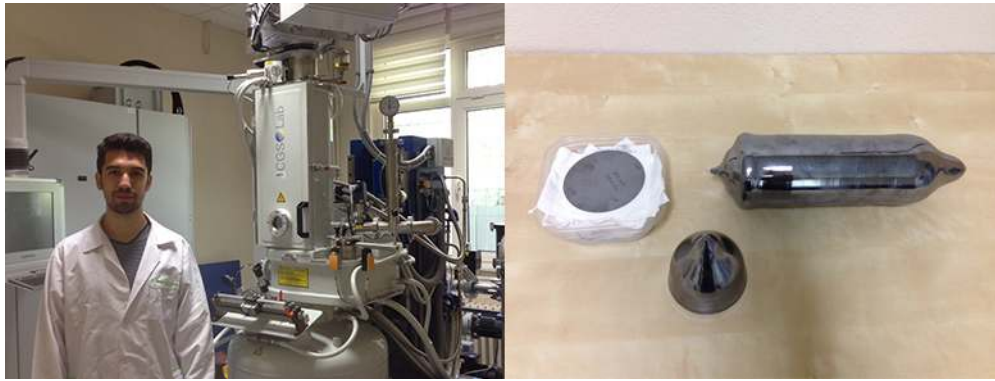
Figure 3.2 Czocharlski single crystal ingot growth machine and produced ingot
