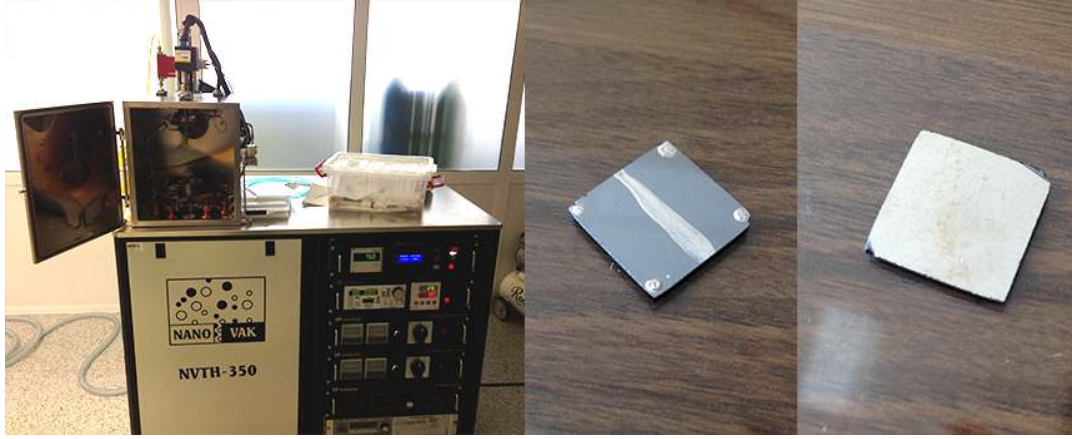
Figure 3.7 NanoVak NVTH-350 PVD equipment and some experiments
