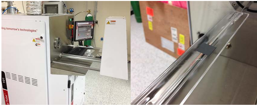
Figure 3.6 CVD furnace and wafer placement
