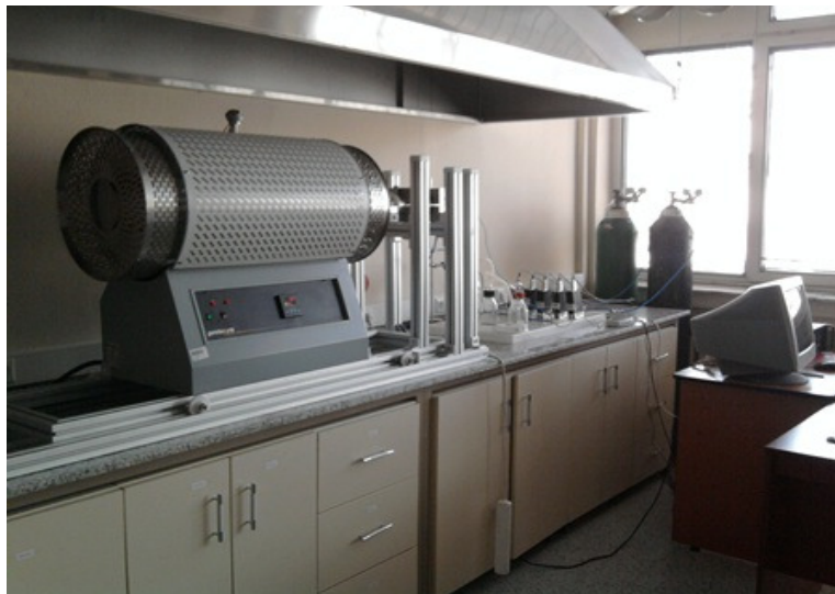
Figure 4.5 Atmosphere controlled heat treatment system.
