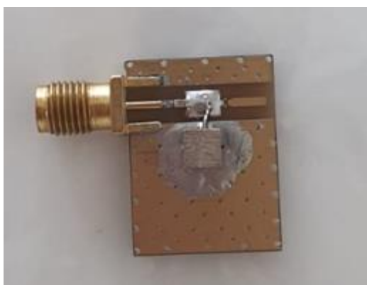
Figure 3.39 CeO 2 -Glass ceramic resonator filter
