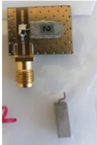
Figure 3.45 0.68\text{CaTiO}_3\text{-}0.32\text{Ca}(\text{Zn}_{1/3}\text{Nb}_{2/3})\text{O}_3 ceramic resonator filter
