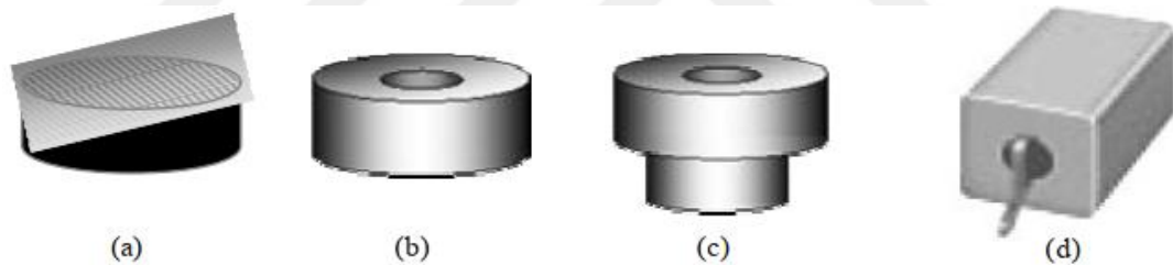
Figure 1.15 Images of dielectric resonators in different shapes; (a) disc, (b) coaxial cylinder, (c) supported coaxial cylinder, (d) TEM mode dielectric resonator [50]
