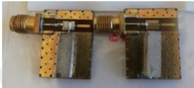
Figure 3.42 \text{Ba}_2\text{Ti}_9\text{O}_{20} ceramic resonator filter
