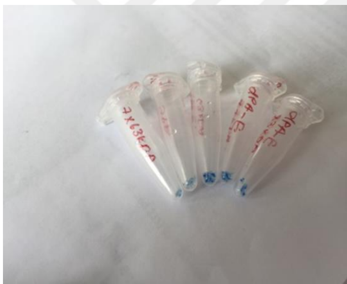
Figure 4.17. The proteins, gel pieces, cut from the gels (Figure 4.16.) for sending to MS/MS
