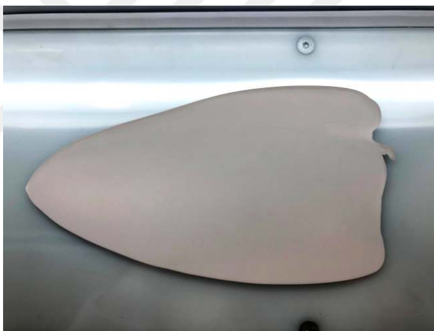
Figure 2.5 Green \text{Si}_3\text{N}_4 tape.
