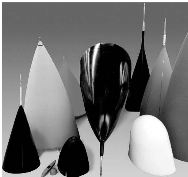
Figure 2.3 Variety of aircraft radomes (Mazumdar, 2001).
