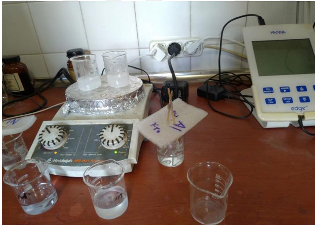
Figure 3.2 Experiment to deposit ZnO thin sheets by SILAR method
