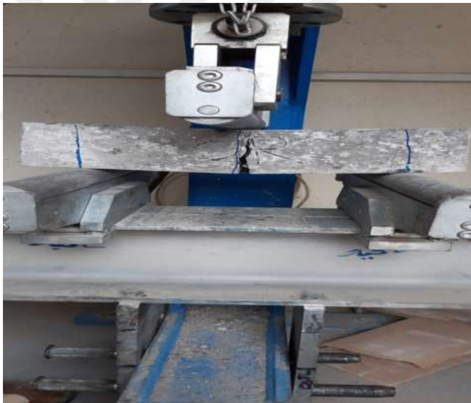
Figure 4.10 Failure mode of plain GHPC
