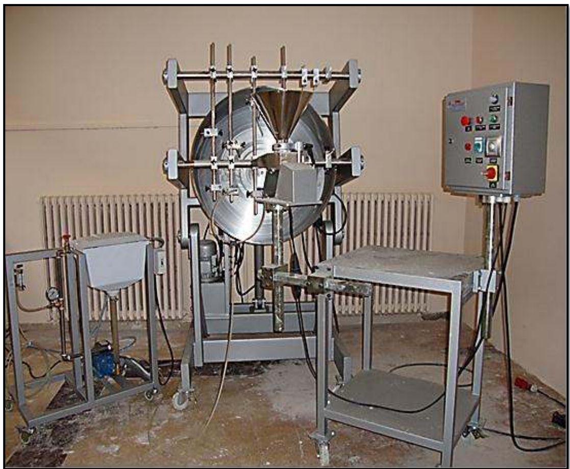
Figure 3.1 The general view of the pelletization disc
