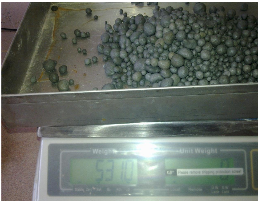
Figure A4 Photographic view of weighted LWA for calculation water absorption
