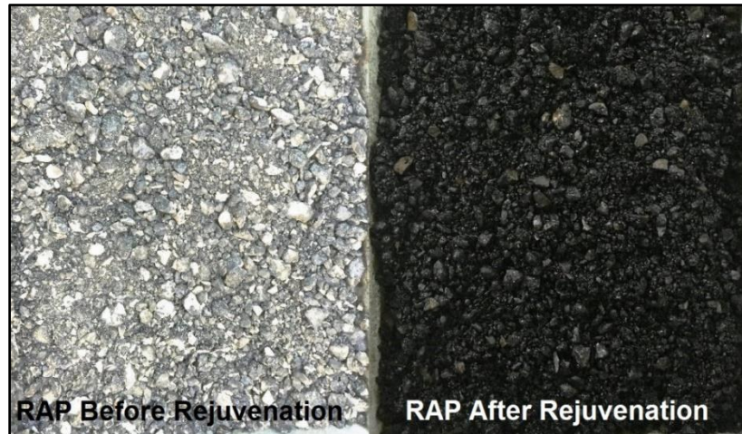
Figure 3.9 RAP before and after rejuvenation (Dokandari et al., 2016)
