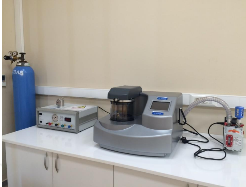
Figure 3.8 Quorum Q150 RES coating device (Katip Celebi University Central Lab., 2016)
