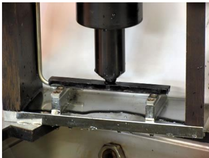
Figure 2.19 BBR beam on its supports (Pavement Interactive, 2012e)
